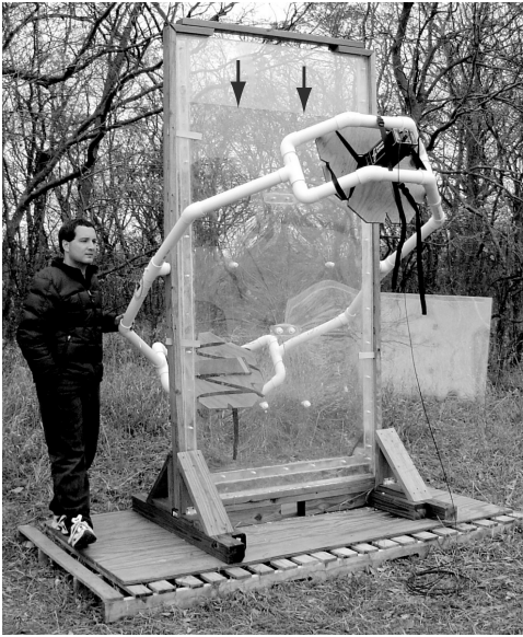
Figure 1. Experimental setting of a simulated fresh-water filled, 4.8 mm aperture thin layer. 200 MHz radar signals parallelly polarized to the thin layer, E-pol, are transmitted at variable angles of incidence ( 0^\circ – 70^\circ ) controlled by the pivoting arm. Rotating both antennas by 90^\circ results in perpendicularly polarized signals impinging to the plane of the thin layer, H-pol. The water level in the simulated fracture is marked by arrows.
