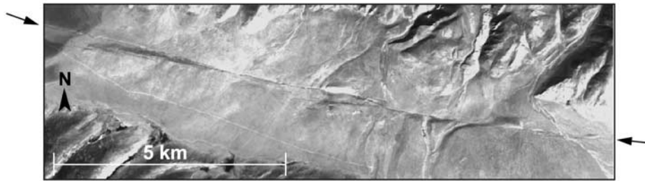
Figure 7. CORONA satellite image of the Gyaring Co fault (arrows) showing fault scarps, pressure ridges, and offset and beheaded streams. Changes in fault strike produce an extensional jog (center) and compressional jog (right), which are consistent with right-slip motion on fault. See Figure 2 for location.
