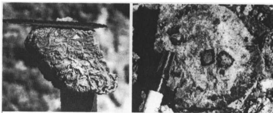
Figure 3. (Left) Concretion with fossils of shells; (right) organic relics in in concretion. Both were found at site 4 during the post experiment ground-truth investigation (pen for scale).
