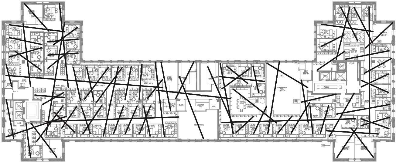
Figure 2: An office layout with its axial map.
