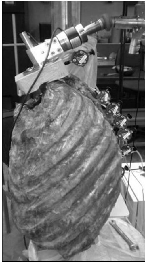
Figure 6.1: Experimental setup depicting a human thoracic spine (T1-T12) with intact rib cage, shown here from the left lateral view. Optical motion-tracking pins are in the top potting of T1 and the pedicles of T6-T10.
