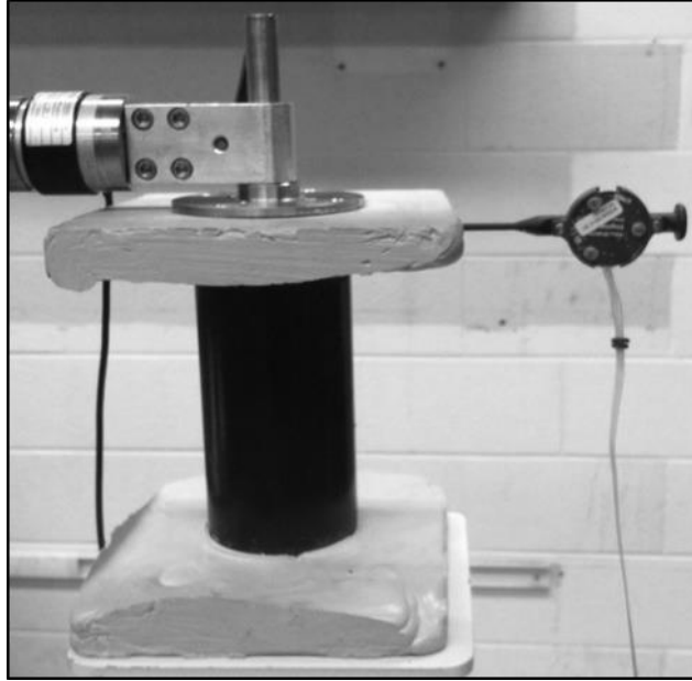
Figure 3.2: Stiff (lumbar) synthetic specimen in bending mode with an optical motion tracking pin inserted to measure actual displacement of the specimen.
