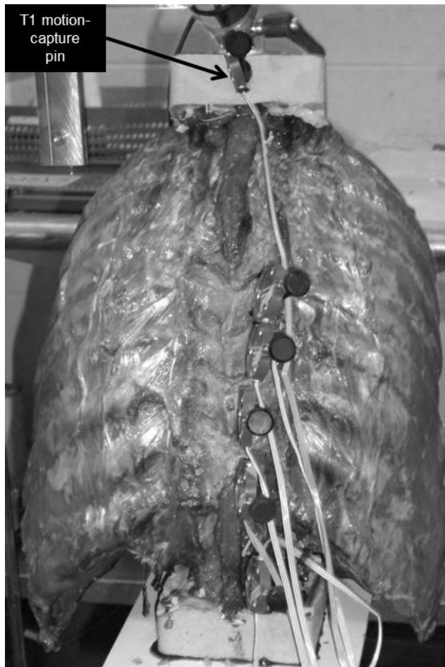
Figure 5.2: Posterior view of testing of Condition 1 (intact rib cage, uninstrumented). The motion-capture pin at T1 was used to track overall motion of the specimen, and the pins at T6 and T10 were used to calculate regional motion between T6 and T10.
