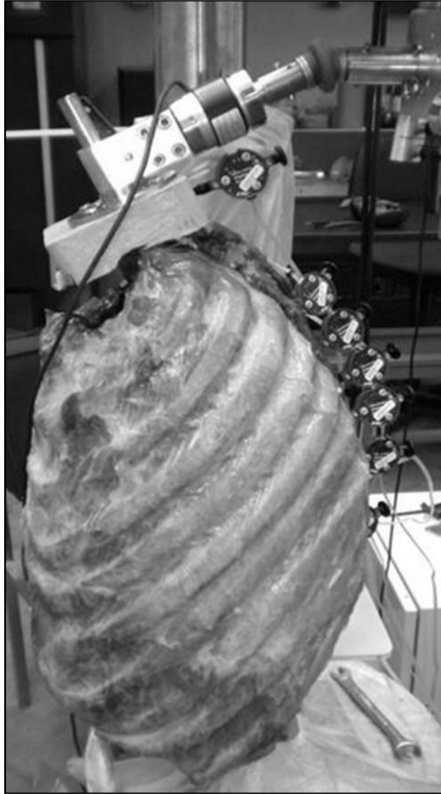
Figure 3.6: Bending test setup of a full thoracic cadaveric specimen with attached ribcage test loaded in the spine test machine
