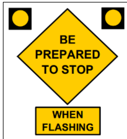
Figure 7 Be Prepared to Stop sign supplemented with flashing beacons (MUTCD, 2009)
