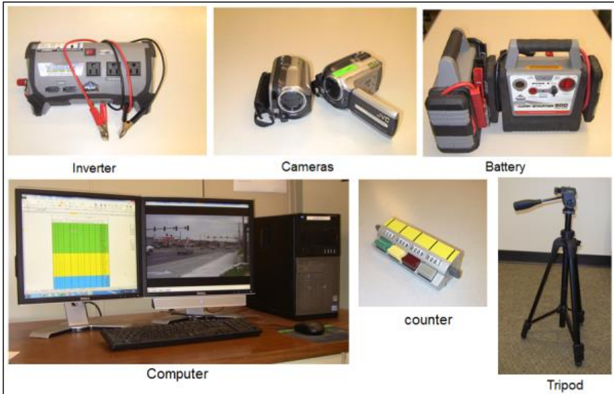
Figure 66. Equipment used for field data collection effort
