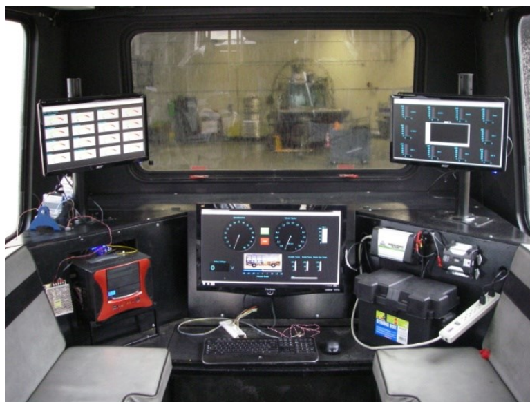
Figure 2.5.1: University of Kansas Shuttle Bus Data Acquisition System
