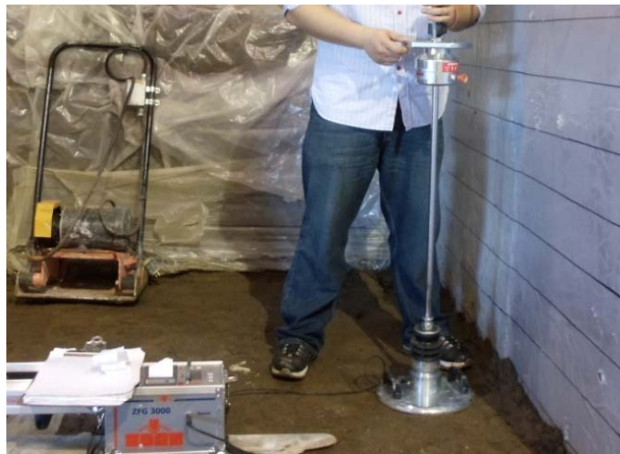
FIGURE 4.26 LWD test on the fat clay
