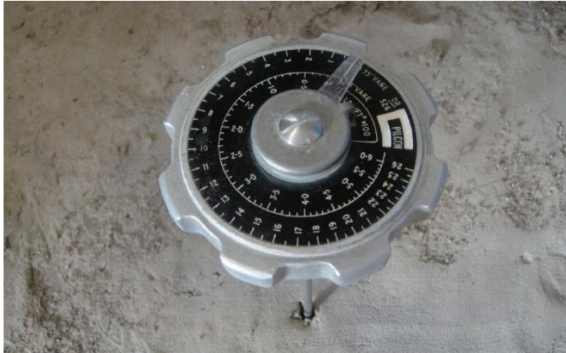
FIGURE 4.25 Vane shear test on the fat clay
