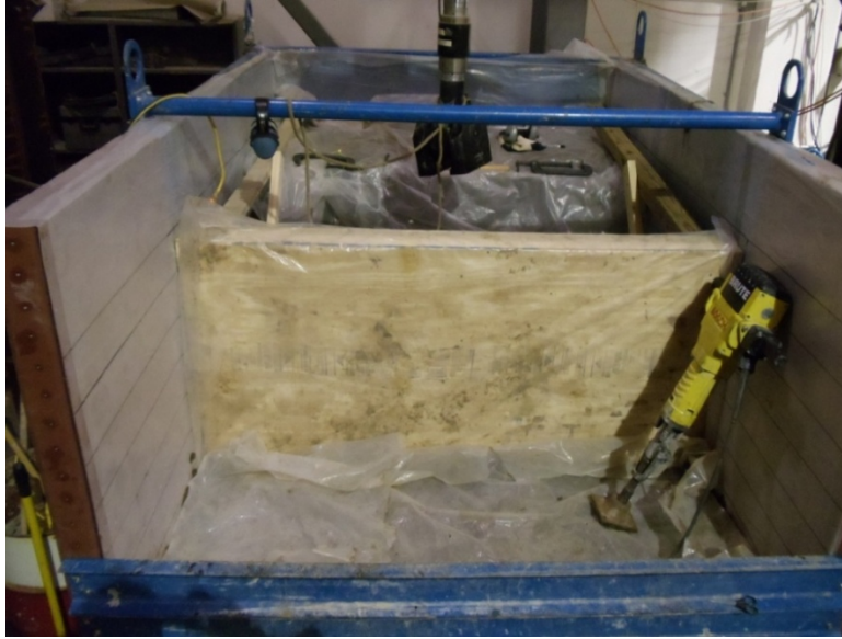
FIGURE 4.15 A polyethylene plastic sheet placed to cover the exposed fat clay
