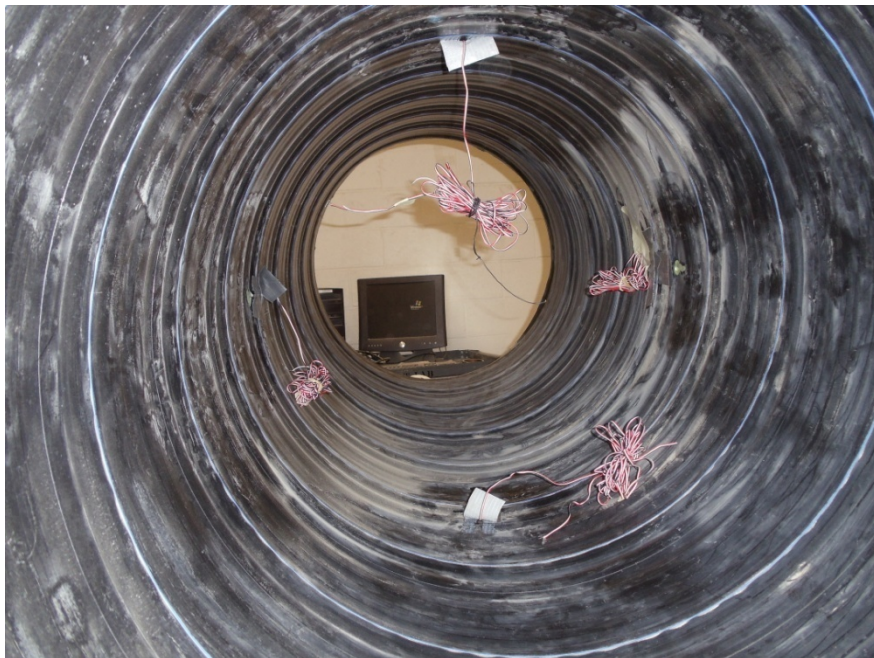
FIGURE 4.9 Strain gages fixed inside of the pipe specimen
