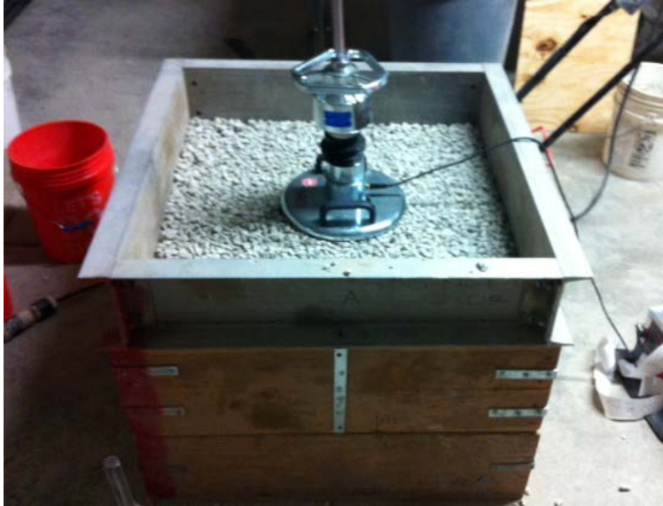
FIGURE 5.32 A small box used for density determination
