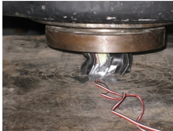
FIGURE 3.14 Specimen crushing in the stub compression test
