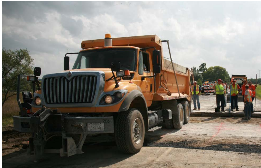
FIGURE 5.23 Test truck used in loading the culvert
