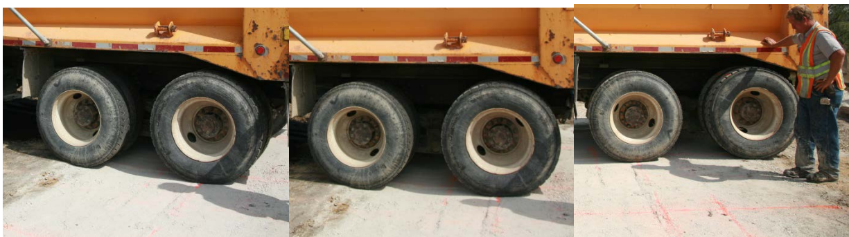
(a) Back tire at the center between the trench wall and the crown (b) Back tire above the crown (c) Middle tire above the crown
