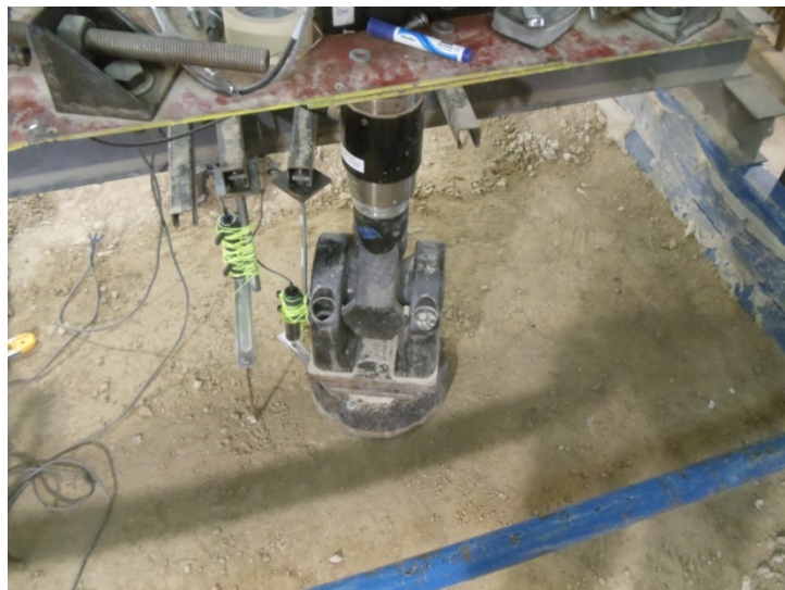
FIGURE 4.28 Displacement transducers fixed to a reference beam
