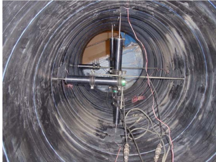
FIGURE 4.5 Displacement transducers inside the pipe section
