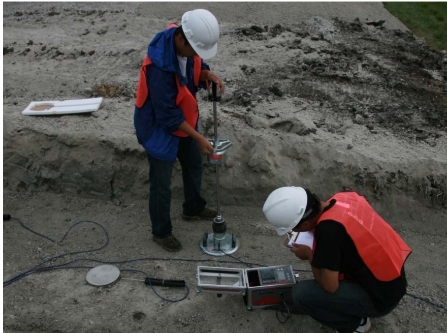
FIGURE 5.30 LWD test on the compacted AB-3-II
