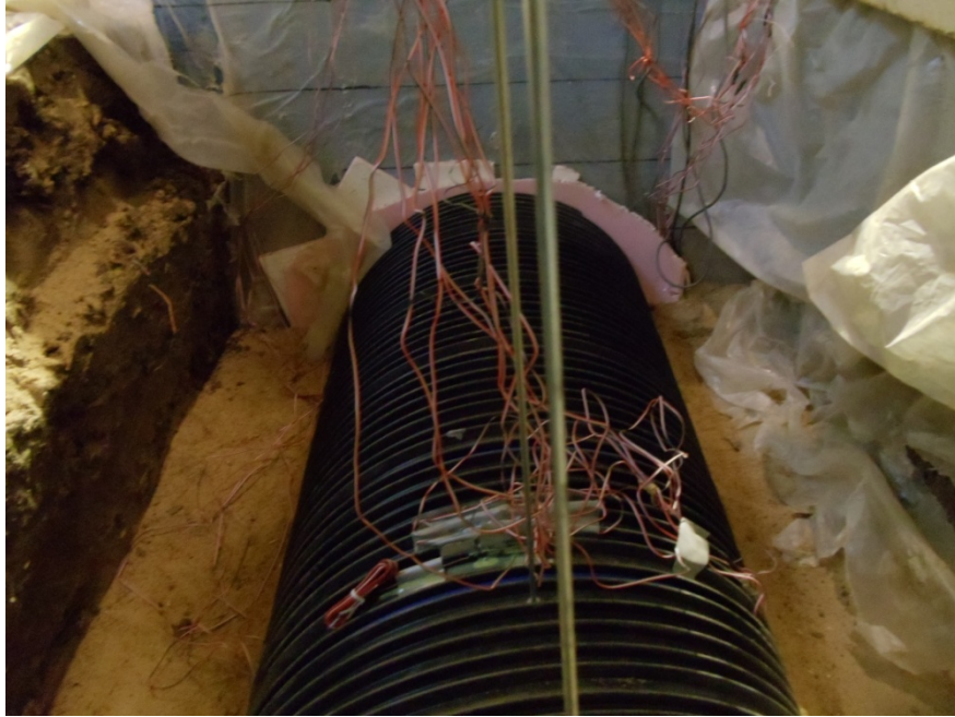
FIGURE 4.6 Tell-tales fixed on the pipe specimen
