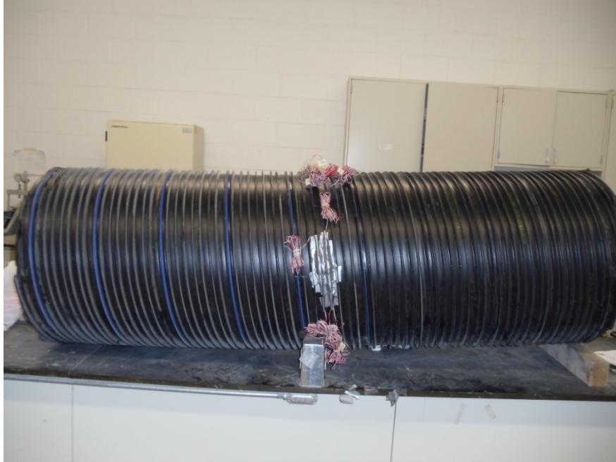
FIGURE 4.8 Strain gages fixed outside of pipe specimen
