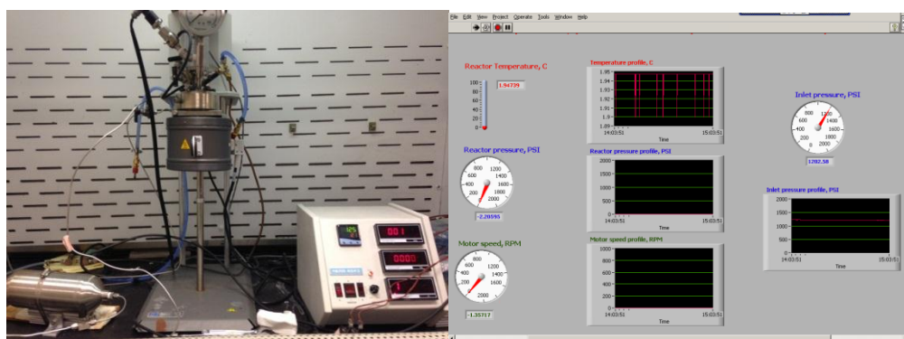
Figure 3. Experimental setup of 300 mL Parr reactor setup (left) and monitoring system (right)
