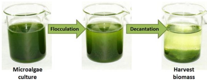
Figure 2.2 Step by step representation of microalgal flocculation (Granados et al., 2012).
