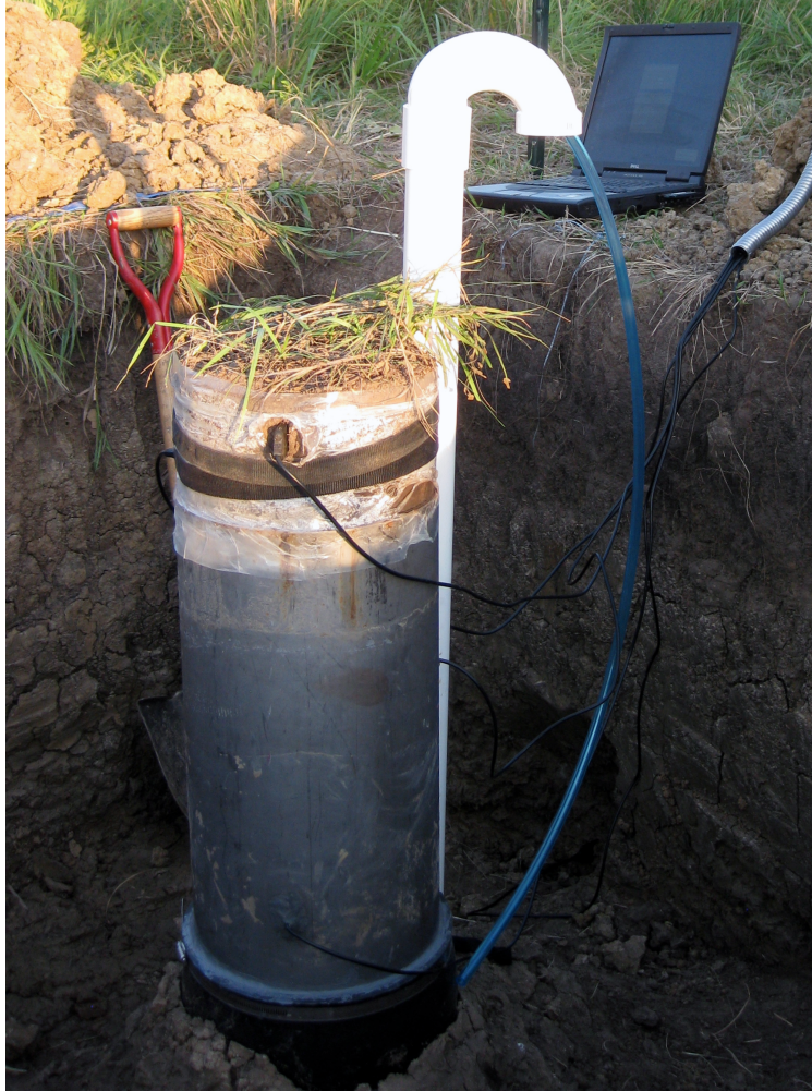
Fig. B8. Passive capillary lysimeter installed at study site, including five soil moisture and temperature probes. The drainage control tube (stainless steel) isolates the natural soil structure below most of the root zone.
