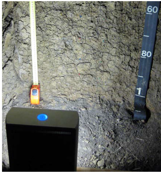
Fig. B1. NextEngine MLT scanner capturing a photograph of the prepared soil pit face just before performing the MLT scan. The yellow measuring tape on the left side of the photo and colored pins inserted in the excavation wall (not visible) provide a reference system.
