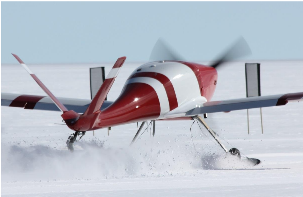
Figure 2.1: Meridian UAS Rudder Deflection (Photo by Dr. Shawn Keshmiri)
