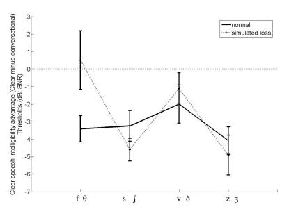
FIG. 4. Clear speech intelligibility advantage (clearminus-conversational thresholds) in dB snr for listeners with normal hearing and listeners with simulated hearing impairment as a function of fricative pair.
