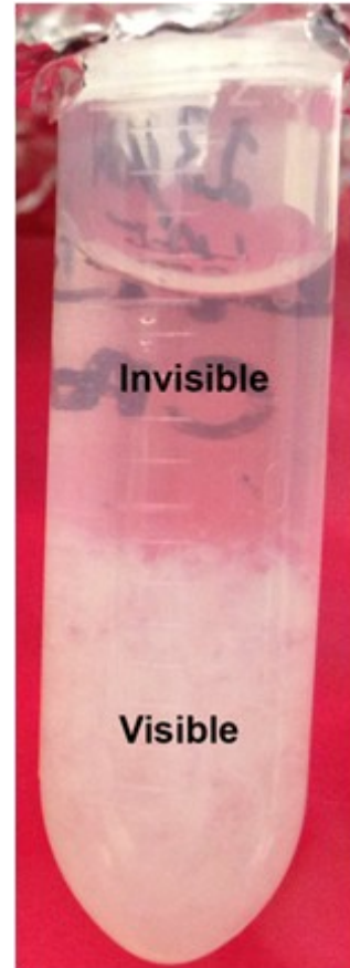
Figure 1. Visible and invisible layers in the sample at the collagen isolation and concentration stage following 24hr incubation in an ice water bath.
