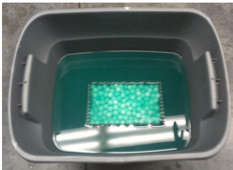
Figure 54 - Catalytic support media immersed in nickel salt bath
