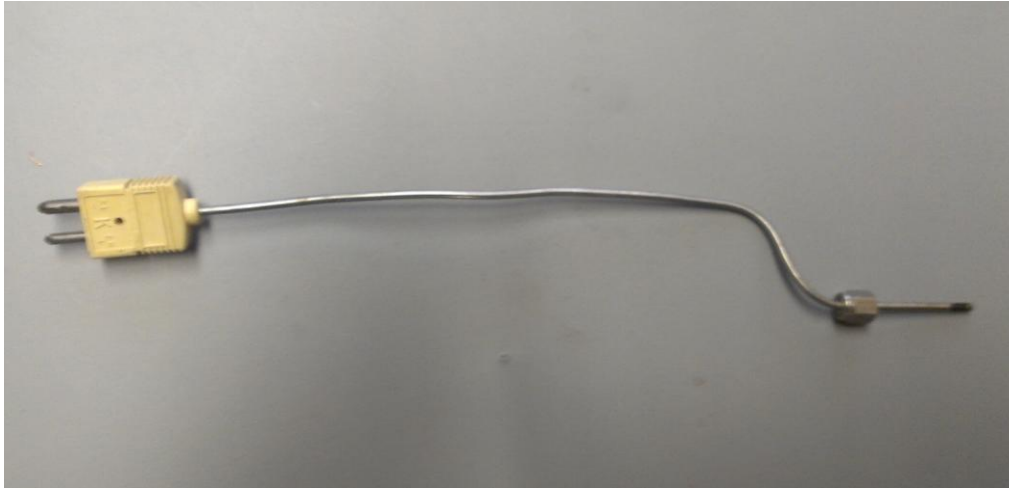
Figure 14 - Standard Omegaclad K-Type thermocouple probe used on the syngas rig
