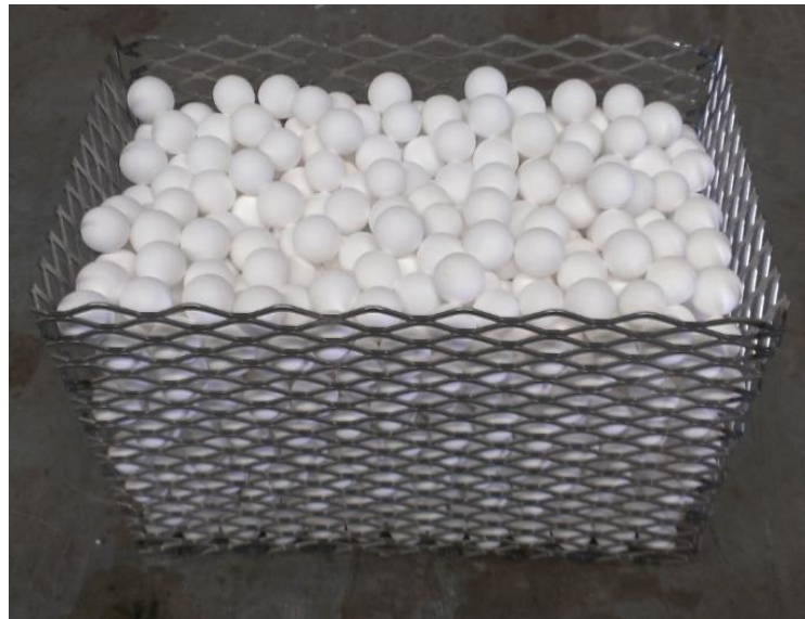
Figure 53 - Catalytic support media before catalyst was introduced
