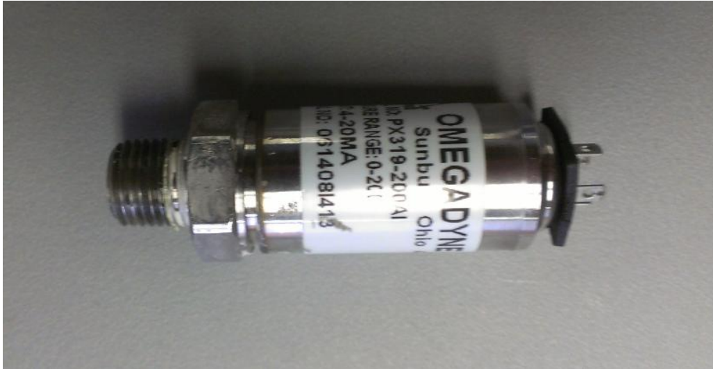
Figure 15 - PX 319 pressure transducer used on the syngas rig
