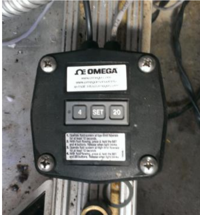
Figure 20 - Glycerin control converter from pulse input to analog input
