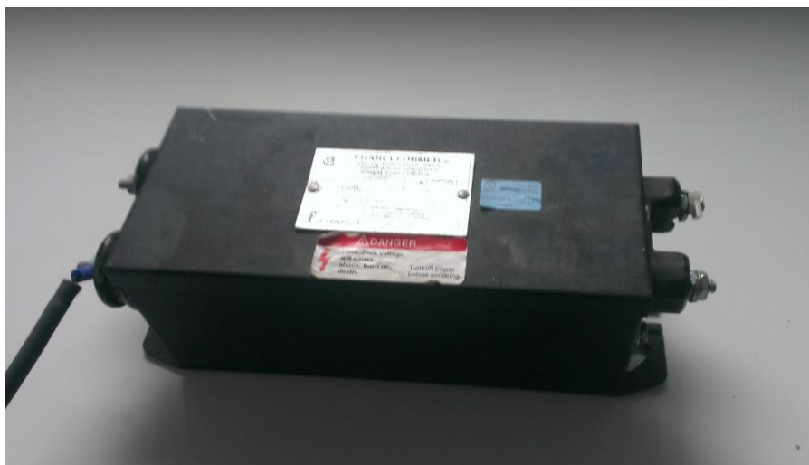
Figure 6 – Franceformer 9030 P4 neon transformer used for spark plug igniter.
