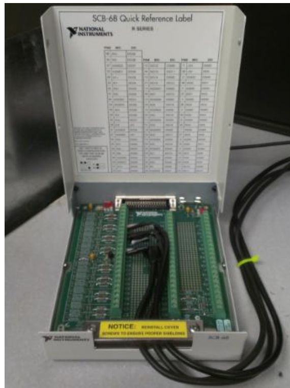
Figure 21 - Shielded input block for in-cylinder pressure measurements
