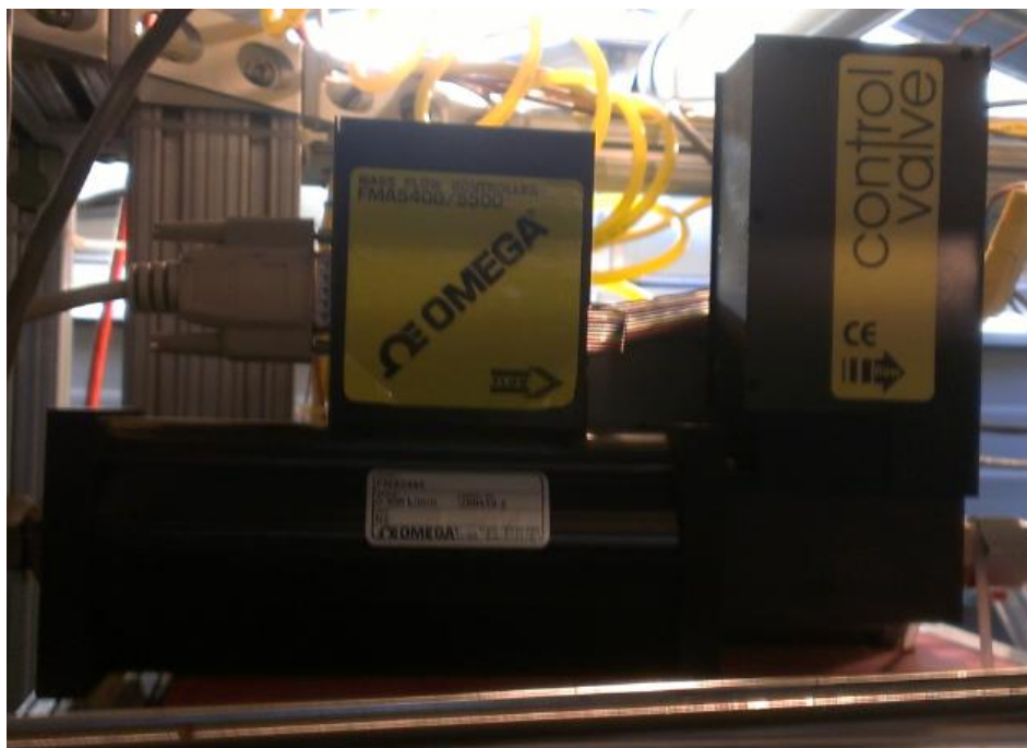
Figure 17 - Omega gas flow controller for propane (or other combustible gasses)
