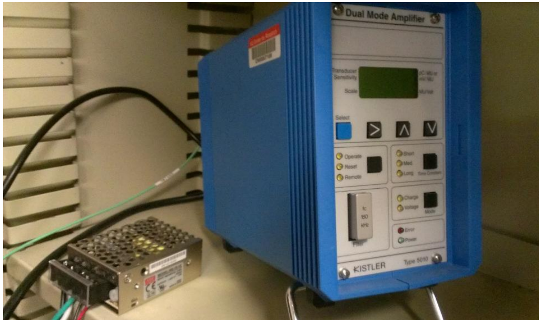
Figure 22 - Power supply (left) and charge amplifier (right) for in-cylinder pressure measurements
