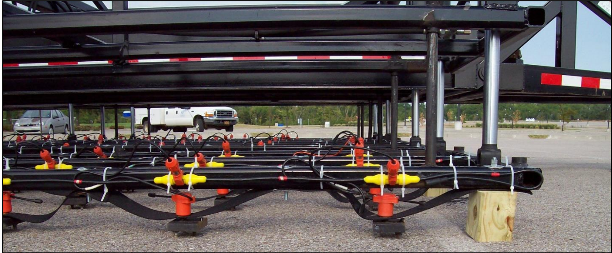
Figure 38. Geophones mounted on base plates. The geophones have been deployed and are ready for data acquisition. While deployed the geophones are not in contact with the Autojuggie and tension has been removed from the nylon strapping.
