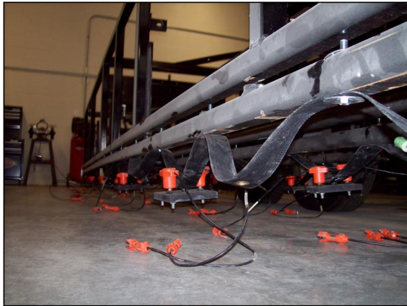
Figure 47. Geophone base plates and nylon strapping. The nylon strapping is secured to the Autojuggie using holes within the lower rung which house spiked geophones when performing surveys on soil
