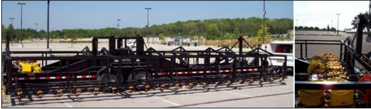
Figure 53. Deploying geophone base plates (left), note the seismographs, cables and batteries on the far left of the image. Close-up view of the recording equipment contained within the Autojuggie during survey (right)
