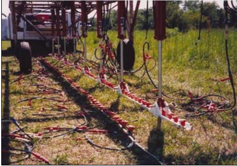
Figure 34 Early autojuggie development. Geophones mounted on channel iron to demonstrate that rigidly attached geophones can accurately record common mid-point data (from Spikes et al., 2005). As shown here, the channel iron is being deployed using a series of hydraulic cylinders
