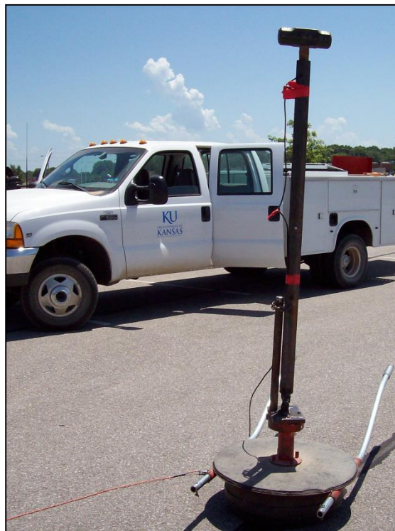
Figure 43. Free-fall seismic source. A heavy sledgehammer is connected at the end of a length of square iron which in turn is connected to the base of a Betsy Seisgun
