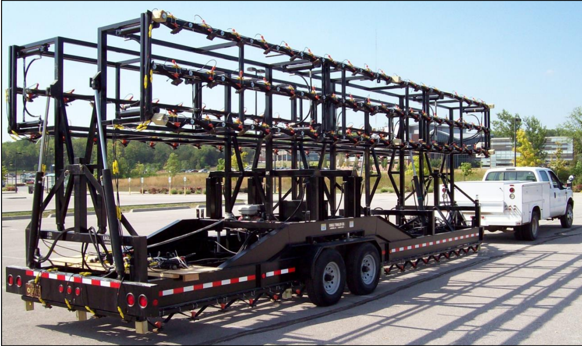
Figure 36. The Autojuggie in its current stage of development. The side wings are in an upright position allowing it to be towed on residential streets
