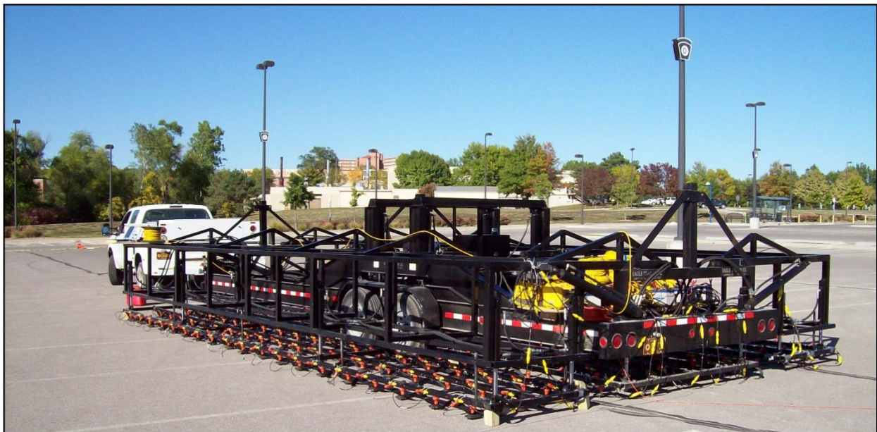
Figure 46. The Autojuggie deployed for marine streamer type acquisition
