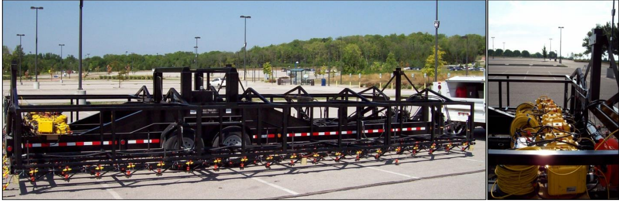
Figure 39. The seismic equipment and cabling remain connected to the Autojuggie when moving the receiver grid to the next position. The seismographs, networking cables and batteries are housed at the rear of the Autojuggie
