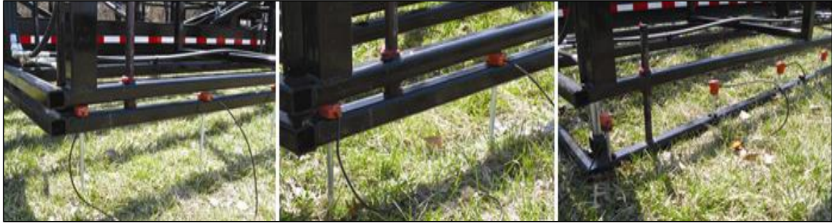
Figure 37. Planting spiked geophones: Before planting begins (left), geophones being planted using the weight of the Autojuggie (middle), separation of the bars leaving geophones free-standing (right) (from Sloan et al., 2009)
