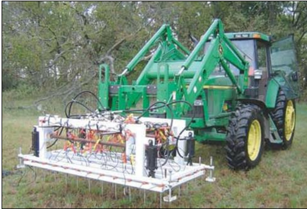
Figure 35. Early autojuggie development. 2D geophone array that could be deployed simultaneously in a 3D survey mode (from Tsoflias et al., 2006). At this stage the geophones were entirely decoupled from the planting device
