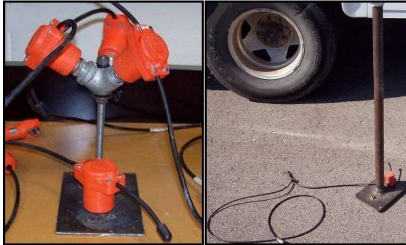
Figure 42. Early base plate design (left) and seismic source (right). Early base plate designs used thin metal for the base with both vertical and Galperin geophones attached. A small sledge hammer is to strike the top of the metal rod
