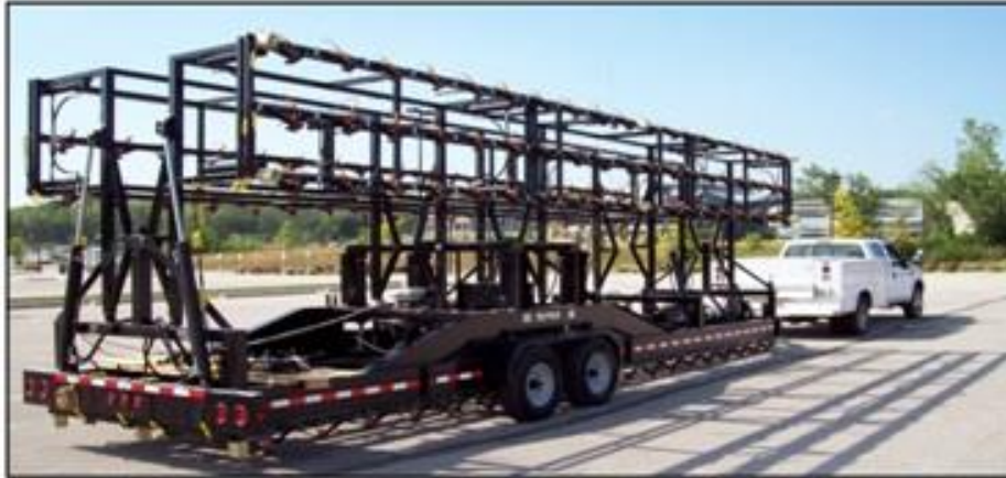
Figure 48. The Autojuggie as it was transported to the field site. Once at the field site only the seismographs, network cables and batteries need to be connected
