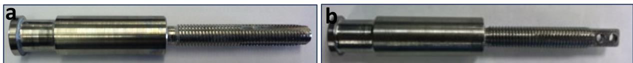
Figure 3.2: a) Endo-prosthesis for pig #1, b) Endo-prosthesis for pig #2. As pictured, the right threaded end of the implant is the side which goes into the bone. The smooth middle section is the transcutaneous piece. The left end with the smaller diameter is the portion onto which the exo-prosthesis is clamped.
