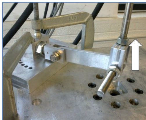
Figure 3.5: Mechanical test set-up for the two-leg hinge joint mechanical test. Tests were run in displacement control at a rate of 1mm/sec over a distance of 10mm.
