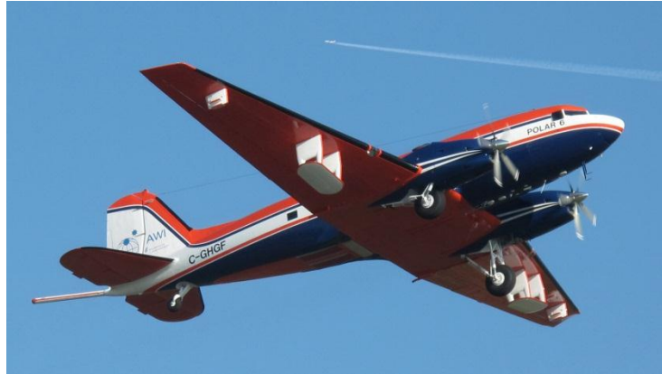
Figure 2.6: AWI Depth Sounder and Accumulation Radar Antennas [41]
