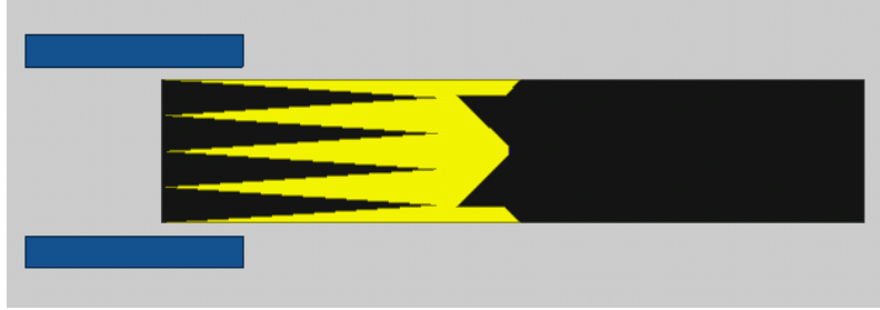
Figure 7.2: HFSS ® Simulation of P-3 Antenna with Ground Plane and Doublers
