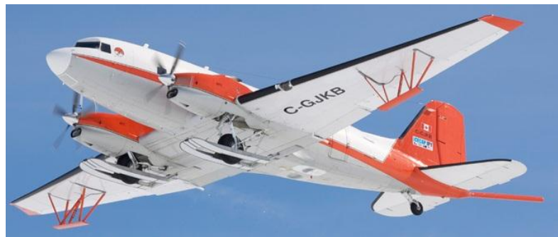
Figure 2.5: HiCARS Antenna Mounted on Basler Wings [38]
