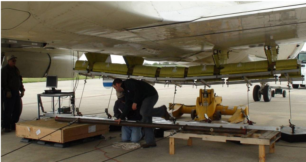
Figure 5.22: Ground Proof Load Test Setup for the Inboard Fairing (photo by Rick Hale)
