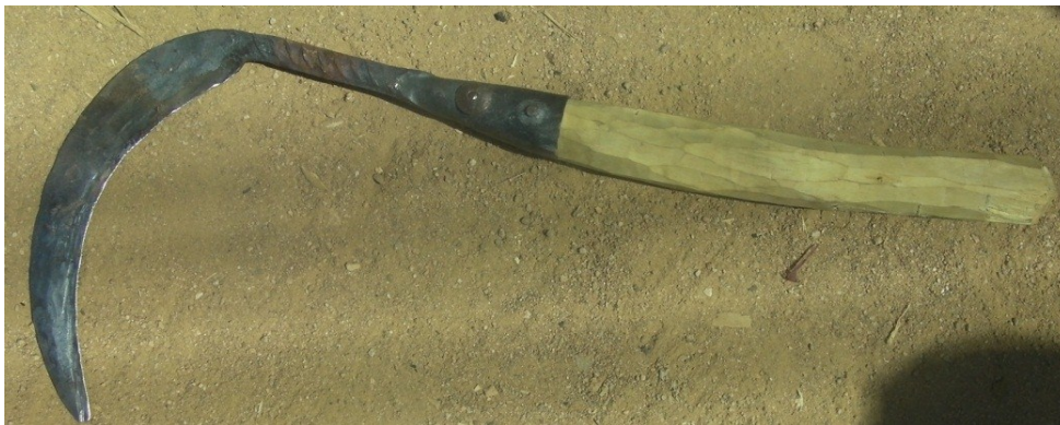
Figure 27: A Typical Sickle used to harvest all type of Grass used in Construction
