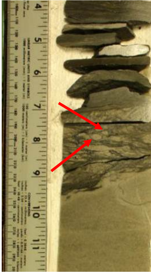
Figure 24: Possible Palaeophycus burrows (arrows) in the Interbedded sandstone and heterolithic mudstone-sandstone lithofacies, Moody D2 core.
