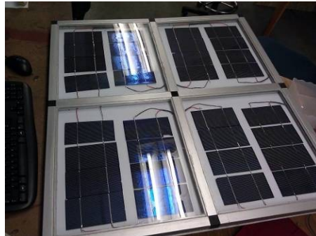
Figure 7: Student built solar panel used to explore solar technology.
