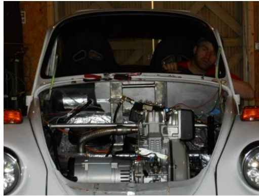
Figure 1: 100% biodiesel generator integrated in a 1974 VW Super Beetle.
