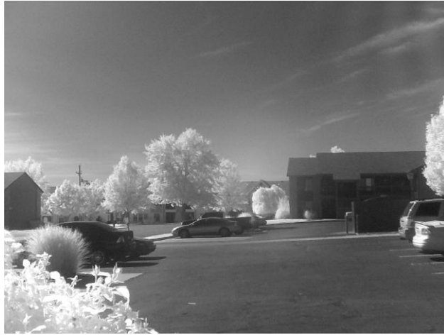
Figure 2. Example of a NIR image taken by the modified BalloonSat camera. The camera was set to record black and white images.
