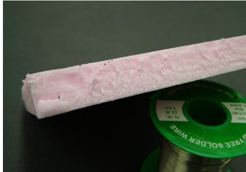
FIGURE 2-9. The edge of Styrofoam cut with a dull blade (A very dull blade was used to emphasize the damage done by a dull blade).
