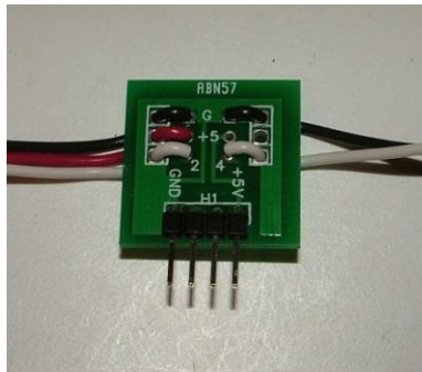
Figure 2. This four pin header has two sensors soldered to it (the sensors are outside the image). Note that the right sensor only has two wires, ground and signal, connecting it to the four pin header. The left sensor is using all three wires, the black wire for ground, the red wire for +5 volts, and the white wire to connection to I/O pin #1 (although the header in this picture says its I/O #2).
