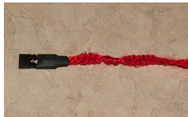
Figure 22. A shorting block sporting a brightly colored ribbon for enhanced visibility.
