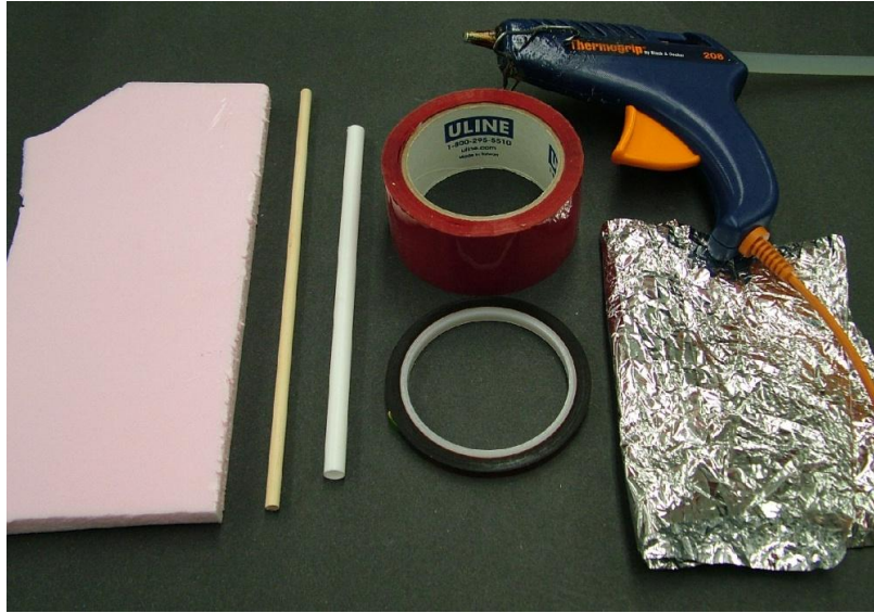
FIGURE 2-13. Half inch thick Styrofoam along with a wooden dowel and hollow plastic tubing. The rolls of tape in the center are a 2.2 mil color coded tape at the top and a roll of Kapton tape below. Both rolls of tape are available from Uline. Kapton is the material used to hold thermal insulation together on real satellites. Space blanket, on the right side, is another covering material for BalloonSats that will help to give yours a real spacecraft look.
