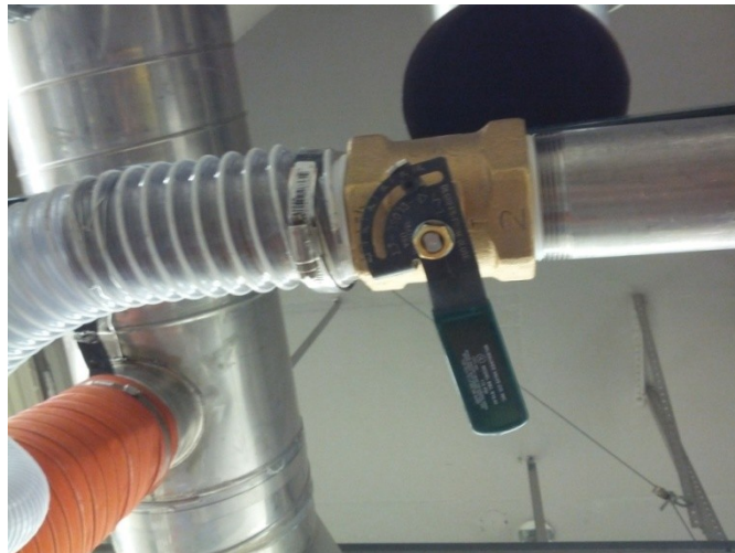
Figure 7. Intake Throttle Valve Downstream of the Laminar Flow Element that Measures Intake Air Flow Rates.
