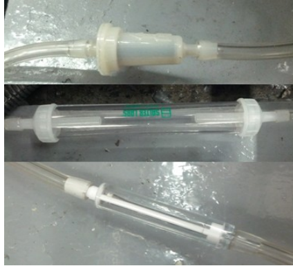
Figure 2. Filtration System for CO 2 Sensors. Top: PM Filter (200 micron), Middle: Water Trap, Bottom: Hydrophobic Filter (0.22 micron).
