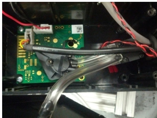
Figure 3. K-33 ICB CO 2 Sensor on the Left with Pump Sensor on the Right.
