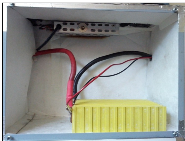
Figure 4: Heated test enclosure with ThunderSky 90Ah prismatic cell.
