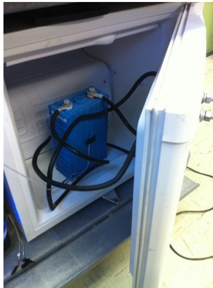
Figure 3: Cold chamber picture of CALB 90Ah prismatic battery inside chamber and connections on outside of chamber.
