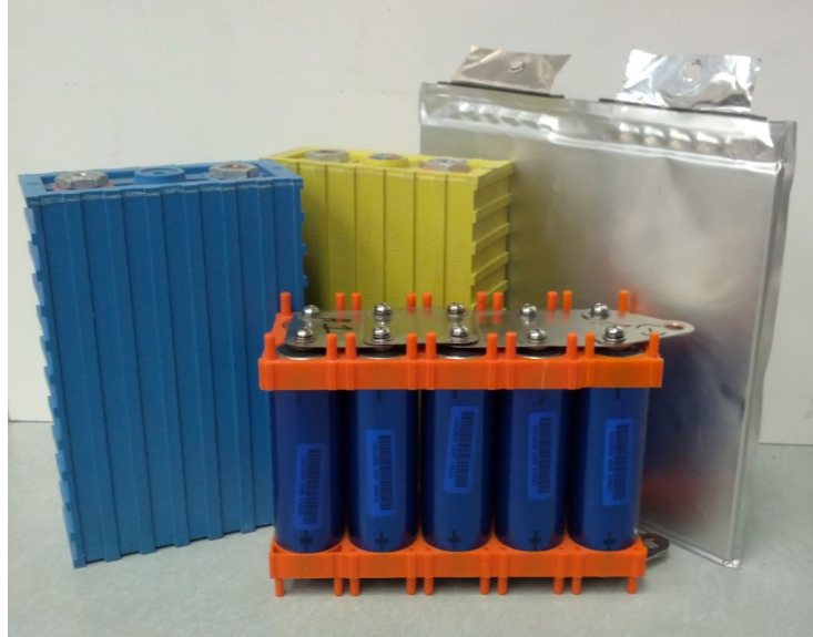
Figure 12: Cells under Investigation (from left to right) CALB 100Ah, ThunderSky 90Ah, Headway 10P1S 100Ah Pack (front), Kokam 60Ah
