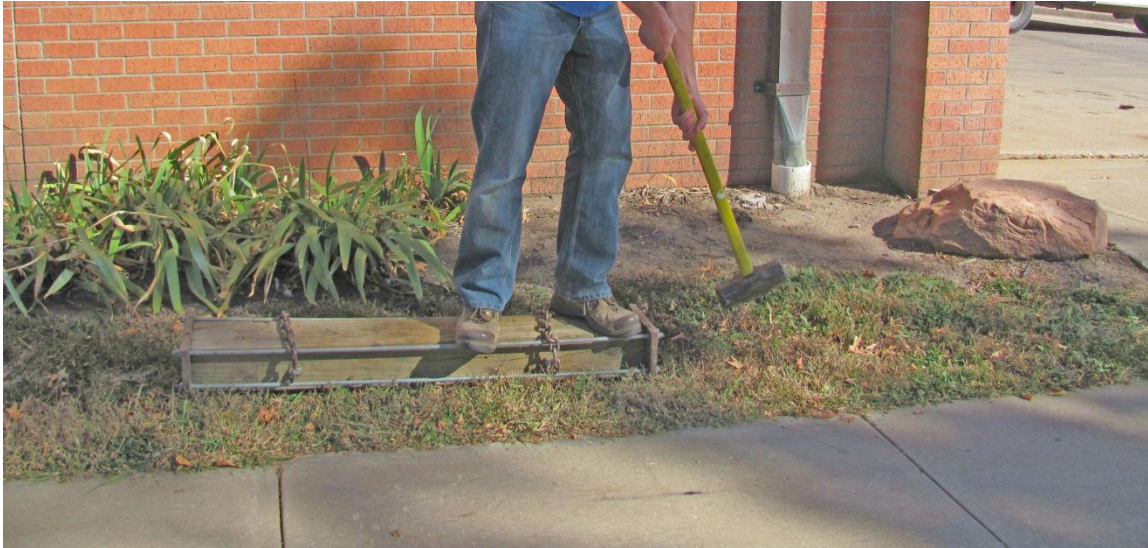
Figure 19: Picture of a shear block used to generate S-waves. The device consists of a block of wood capped with steel plates with teeth for gripping the earth on both ends. Either end of the block is struck to generate S-waves. The person swinging the hammer stands on the block to improve coupling and reduce the risk of inelastic deformation.
