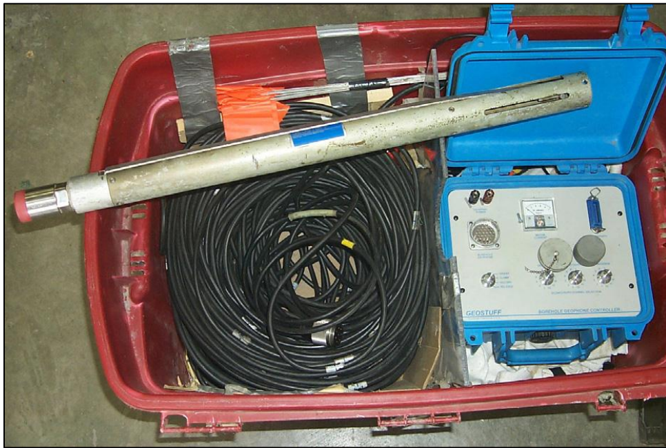
Figure 29: Image of the Geostuff brand three-component downhole geophone (10 Hz) with Kevlar cable and controller used for this survey.
