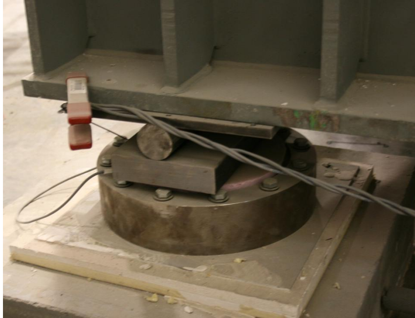
Figure 3-2: Load cell at girder support
