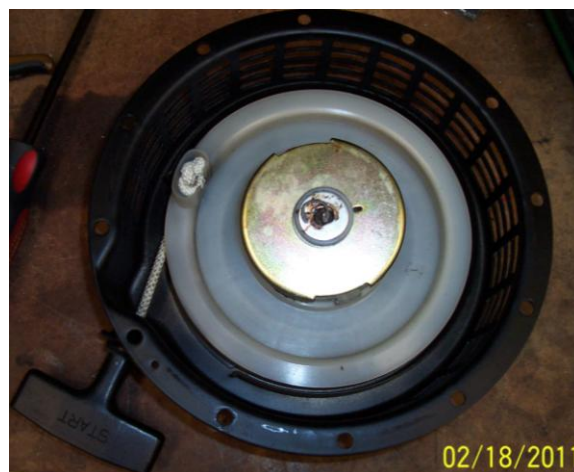
Figure 15. Yanmar Pull-Rope Starting Mechanism Disassembled from Engine
