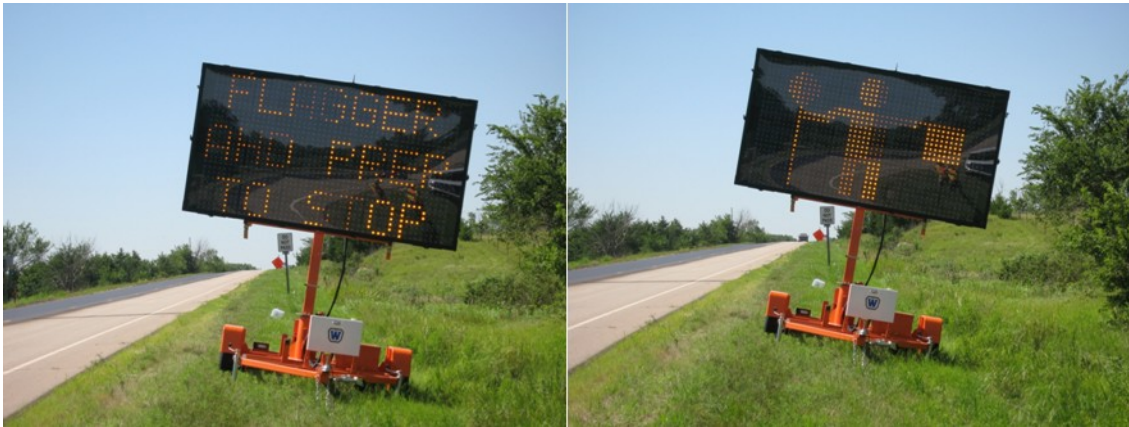
Figure 4.6 Text-graphic PCMS with the Flagger Graphic
