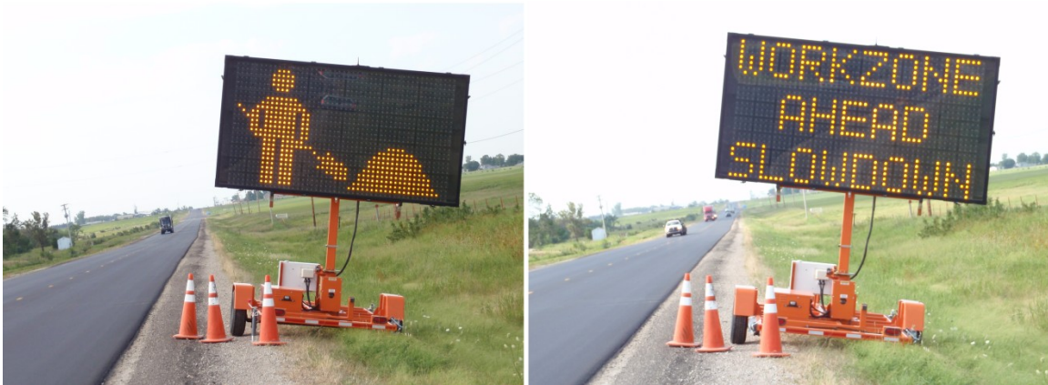
Figure 5.4 Text-graphic PCMS Alternative Two
