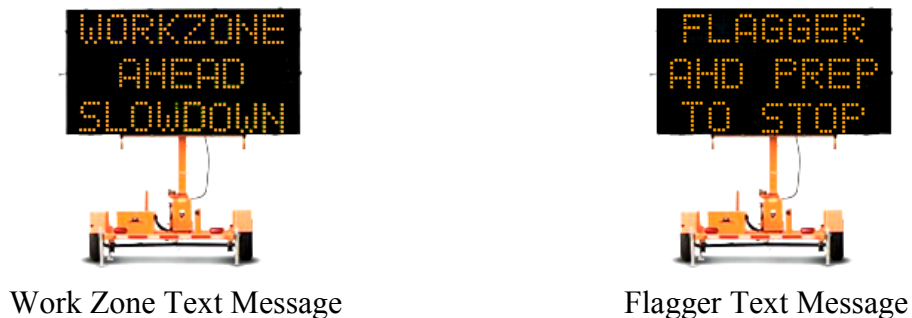
Figure 4.1 Text Messages Displayed on PCMS
