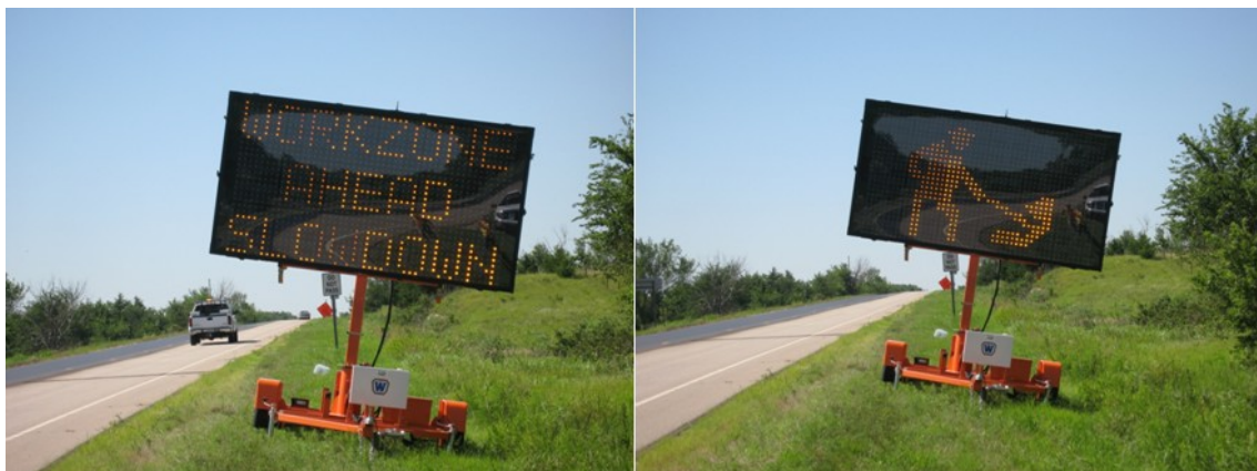
Figure 4.5 Text-graphic PCMS with the Work Zone Graphic
