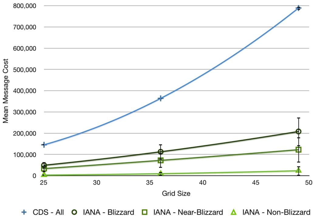
**Figure 28.** Message Cost Means and Standard Deviations.
