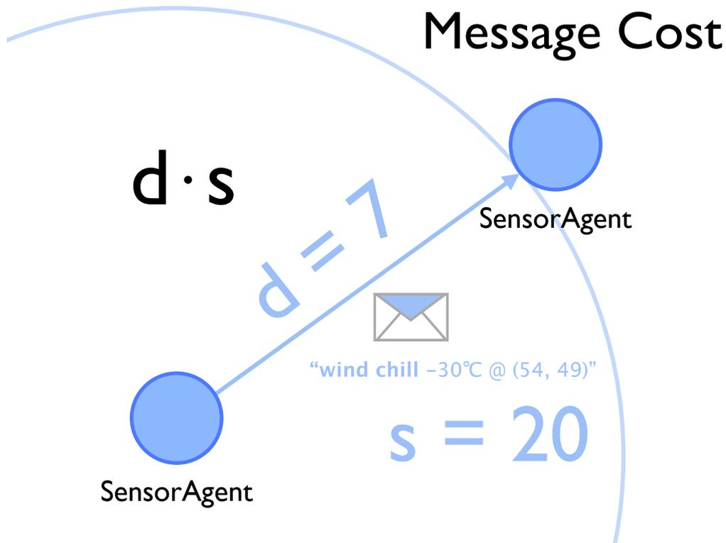
**Figure 20.** Message cost is calculated as the distance of communication times the length of the string communicated.
