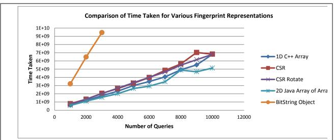
**Figure 10.** Results of the querying a bit bound pruning index when various fingerprint representations are used. The line representing the BitString Object is truncated due to rapid increase in time taken.
