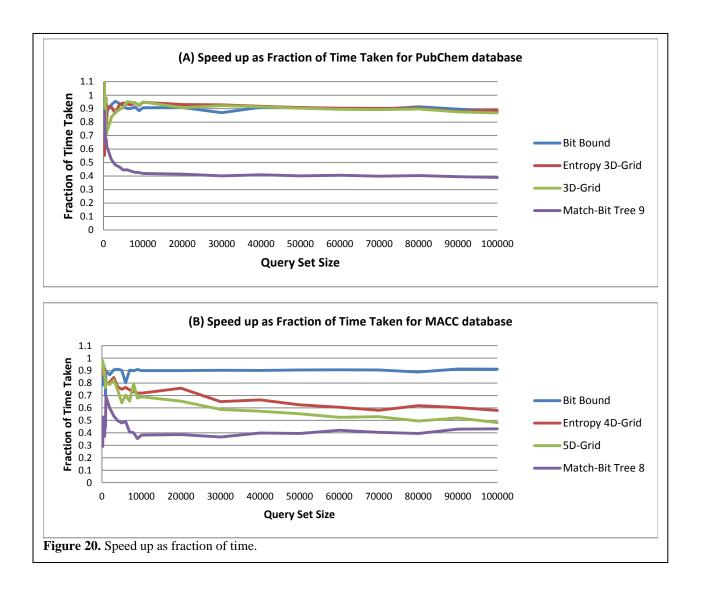
Additionally, Figure 20 shows that nearly any sized batch query larger than 100 query fingerprints receives some sort of improvement. In the case of bit bound, its ability to prune well for very small sizes is evident as *k*D-grid descends from 1 while bit-bound and match-bit tree ascend to a maximum before descending again.
