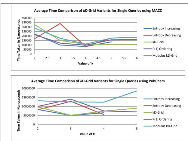
**Figure 11.** The average amount of time taken to run a single query from each fingerprint database is shown here. The experiment was performed 10,000 times with a 0.9 similarity threshold using a random non-repeated fingerprint for each value of k and then averaged. For values of k not powers of two, the segmentation patterns resulting in the best pruning were selected.
