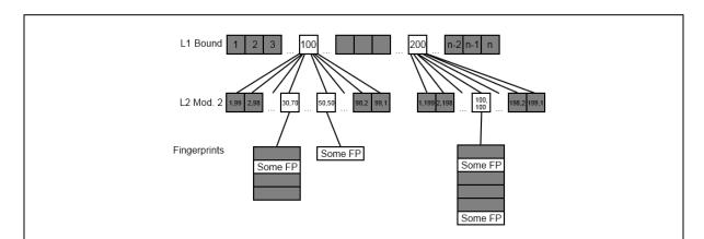
**Figure 16.** This shows an example search index being pruned for an exact search using the query set presented in Figure 15. Grayed out sections are pruned while white sections are unpruned. A search using single queries would take a maximum of query set size (4) multiplied by number of hashes each (2) or 4\*2 = 8 pruning steps. A search using the SimDex batch query set index would only take total number of distinct hashes or 5 pruning steps.
