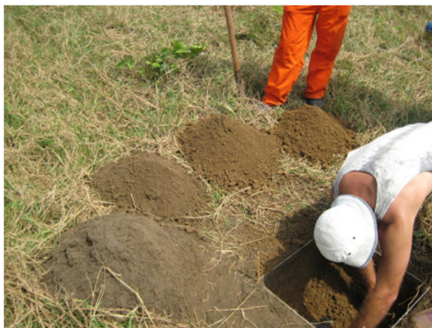
Figure 8 - Test pit aperture to collect bulk density samples
