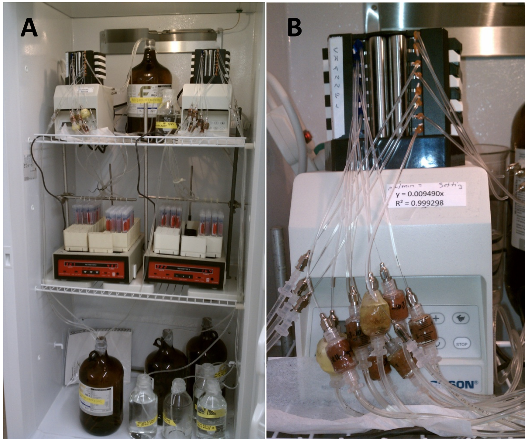
Figure 14 – [A] Pump setup - influent arsenic solutions connected to pumps connected to sample collector; [B] Close-up view of filters connected to Minipulse 3 peristaltic pump (Gilson)
