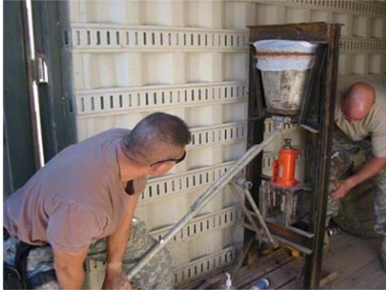
Figure 4 – Operation of a hydraulic filter press (Potters for Peace 2005)
