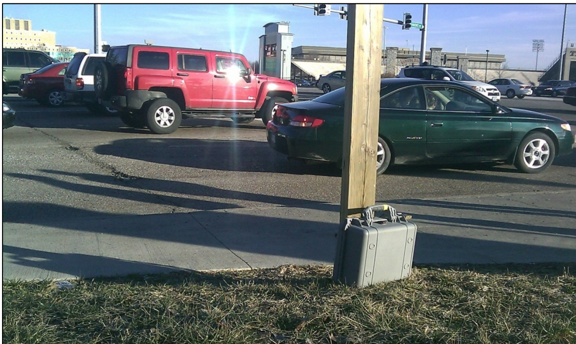
Figure 22 Bluetooth data logger placement at Providence Road and Stadium Boulevard intersection.
