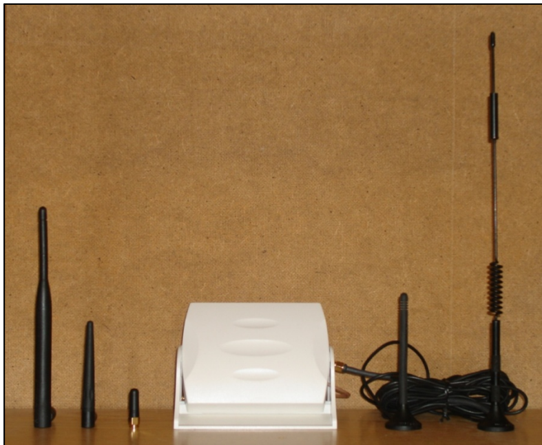
Figure 11 Testing antennas, left to right: 5dB dipole, standard 3dB dipole, 1dB stub, 9dB patch, 3.12 dB whip, 6.12 dB whip.
