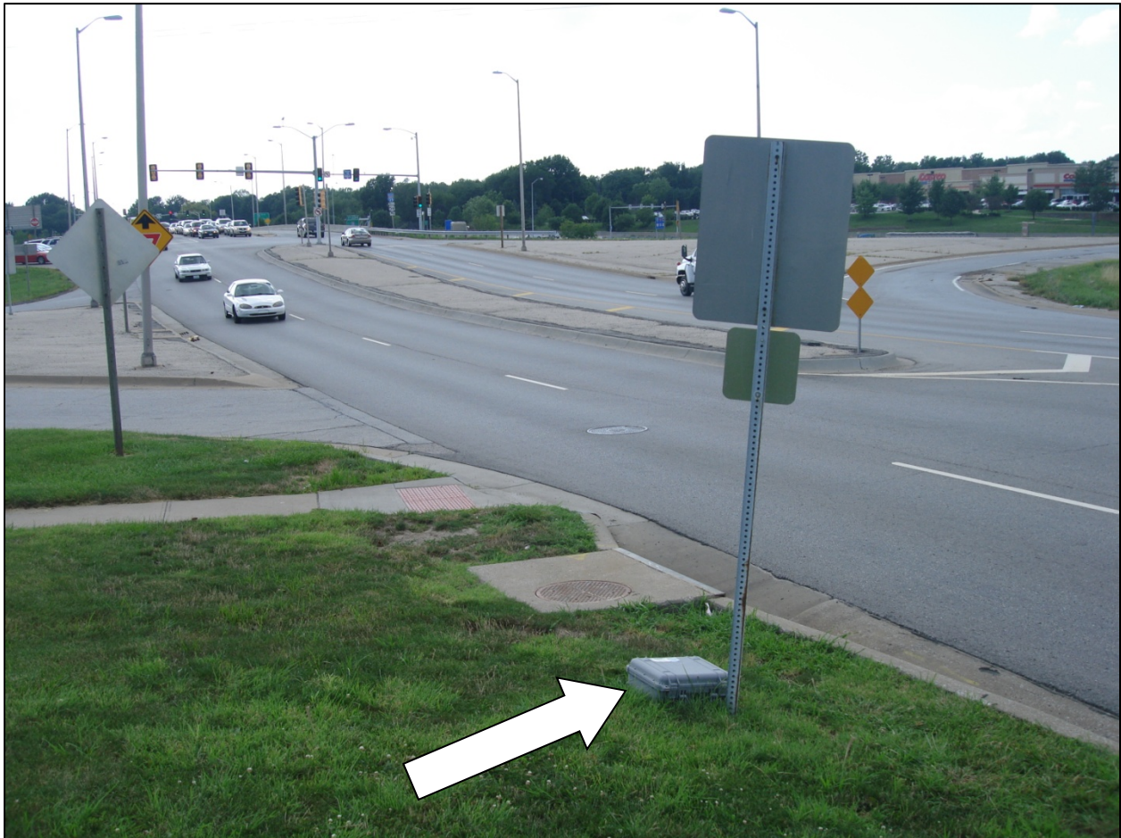
Figure 17 Bluetooth data logger at the northwest corner of I-35 and 95th Street in Lenexa, Kansas.
