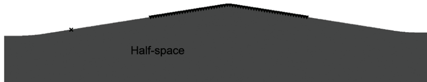
Figure 3-1b. A homogeneous half-space earth model whose free surface is a ridge. The cross indicates the location of the point source. The triangles represent receivers. The center of the receiver array is exactly located on the peak of the ridge.
