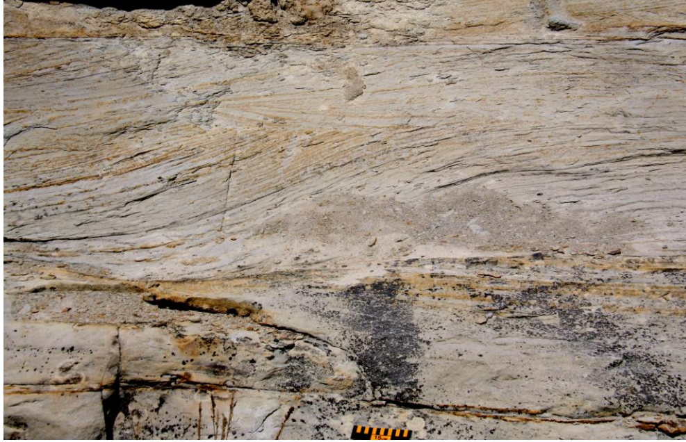
Figure 10. Cross-stratified sandstone exposed in Corcoran Mine. The sloping surface of the outcrop exposure gives the cross-stratification a large apparent thickness. The true thickness of the cross-stratification in this locality is approximately 20 cm (15 cm scale at the base of the photo).
