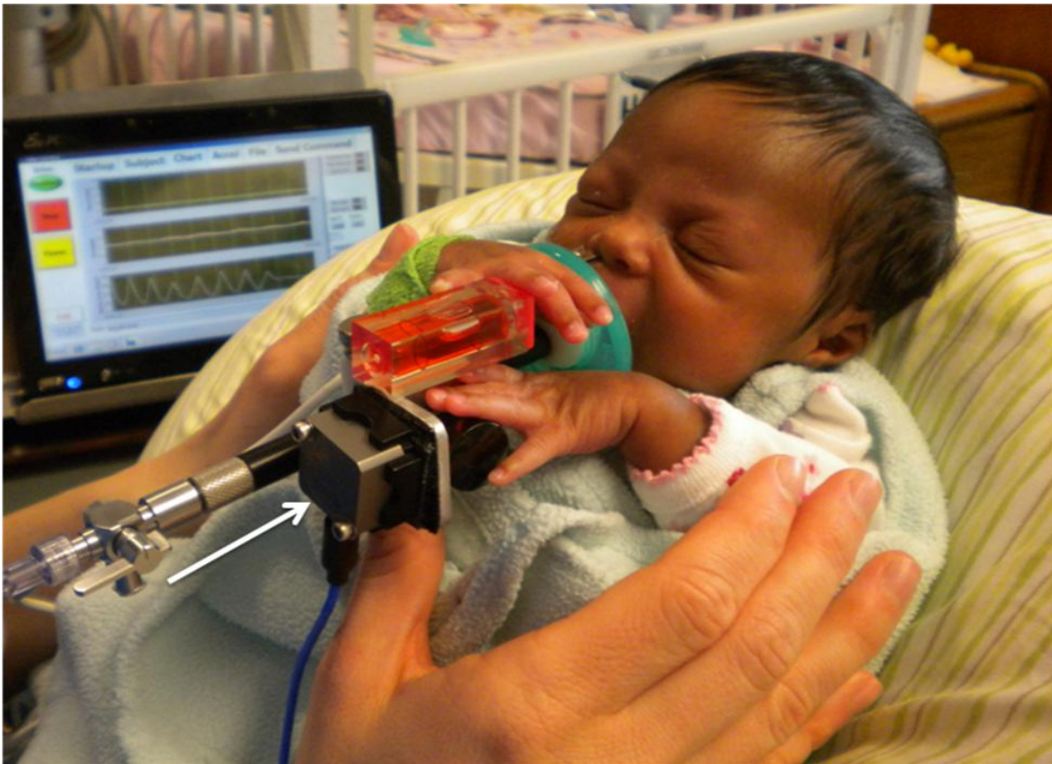
Figure 12: Accelerometer (white arrow) and line mount (red) mounted on infant's pacifier receiver.
