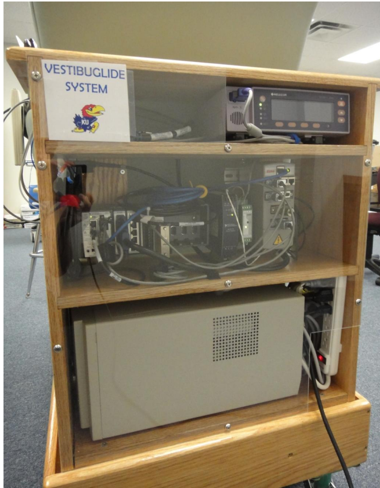
Figure 10: Back of the VestibuGlide chair. Upper right: NELLCOR OxiMAX™ N-600 Pulse Oximeter , middle shelf: cRIO FPGA and motor controller, bottom shelf: isolation transformer and power on/off switch.
