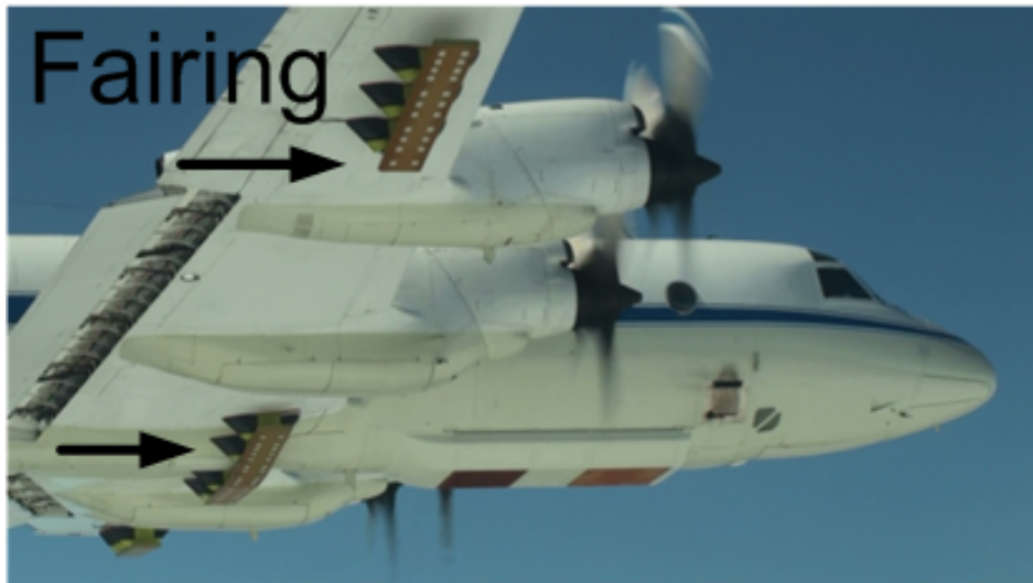
Figure 1.1: Custom Aerospace Fairings Enclosing Radar Antennas on a NASA P-3 Aircraft
