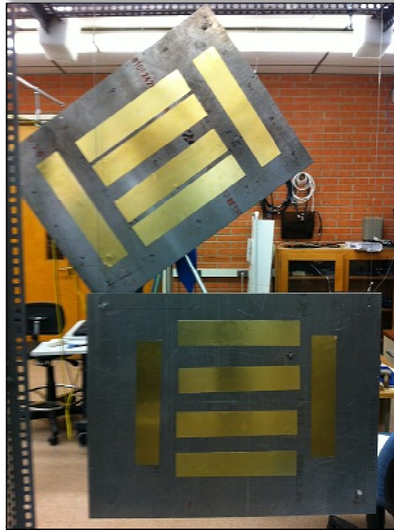
(b) 6 sheets of damping
