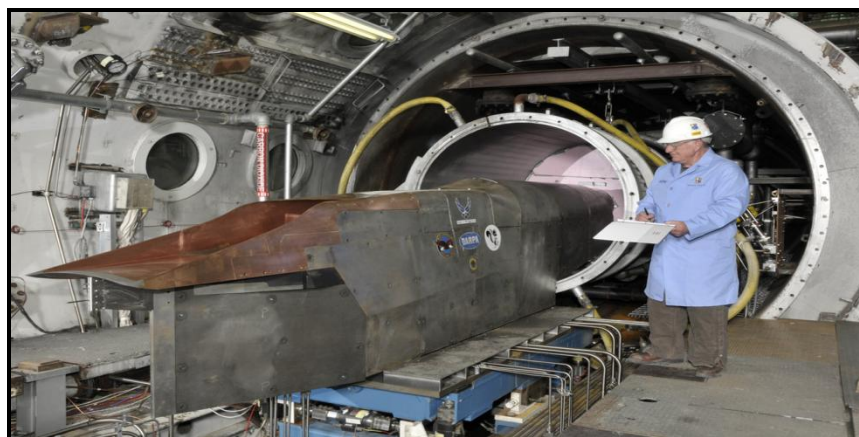
Figure 23: DARPA's Falcon Combined-cycle Engine Technology (FaCET) scramjet test article in the APTU's Test Cell at AEDC [29]
