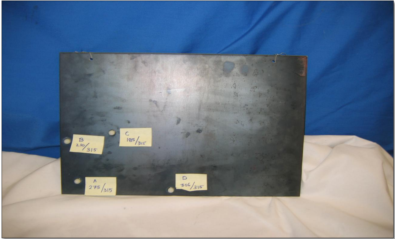
FIGURE 1-14 UNDAMPED STEEL PLATE
