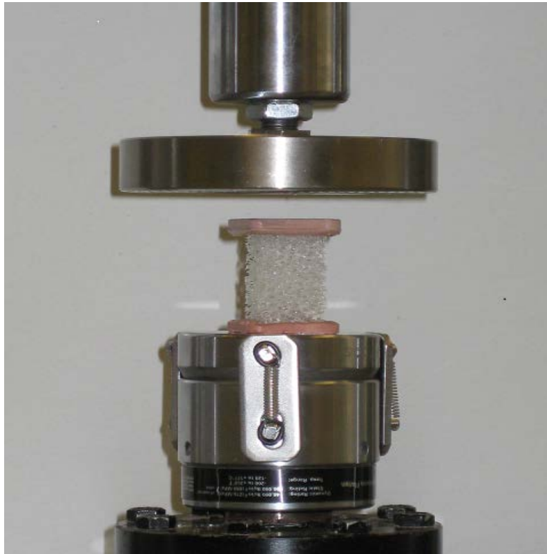
Figure 35: Experimental foam compression test setup. The lower platen is self-aligning, and the ends of each material were potted with filled polyester resin to prevent end artifacts.
