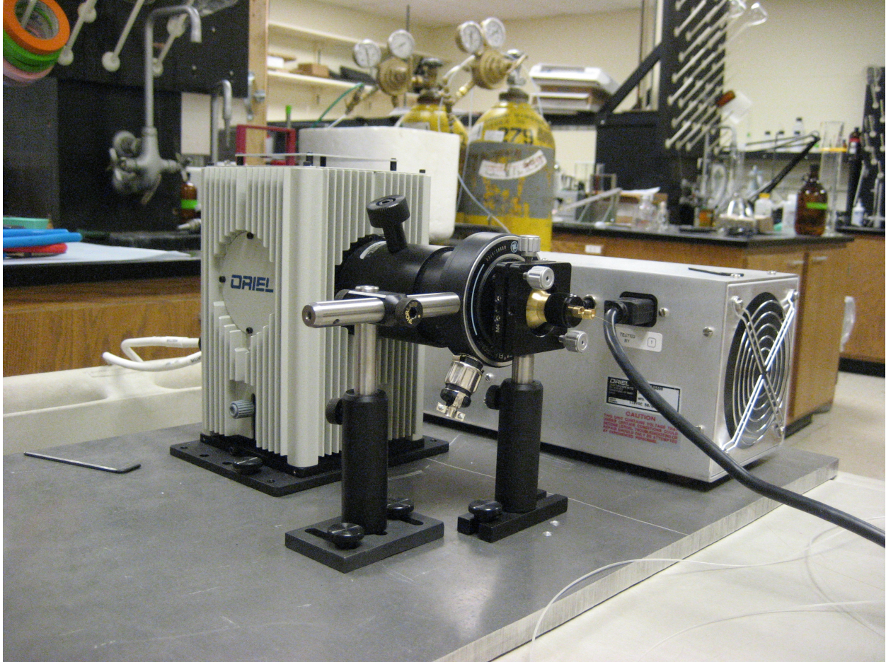
Figure 3. Mercury lamp with the shutter and fiber optic set up in front of the lens.
