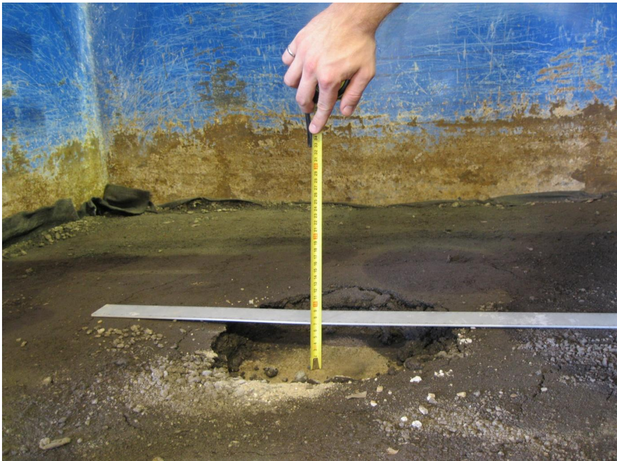
Figure 5.2.6 Displacement measurement at the end of a cyclic plate load test
