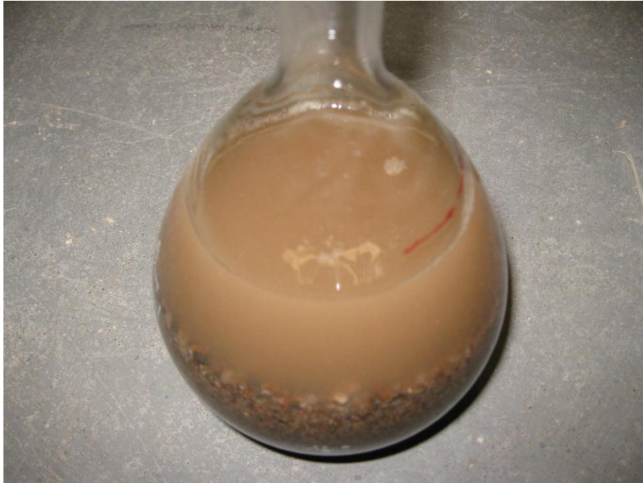
Figure 3.2.10 Pycnometer after removal of air bubbles
