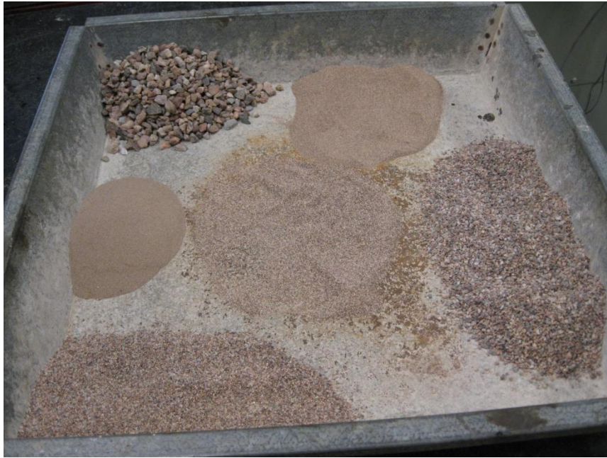
Figure 3.2.5 Fractions of aggregates obtained by sieve analysis
