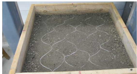
Figure 4.2.6 Multi geocell-confined and embedded
