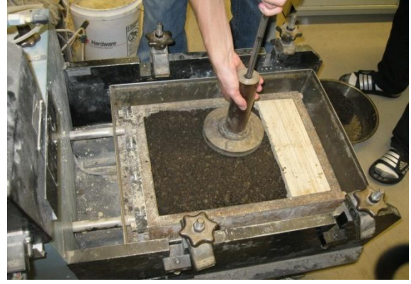
(b) Placing RAP inside the lower box and compacting
