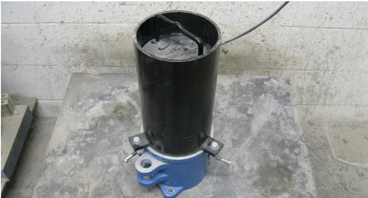
(d) Placing the surcharge weight on the surcharge base plate and then applying vibration
