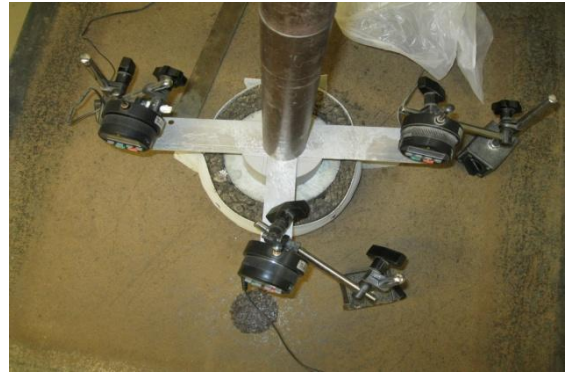
Figure 4.2.4 Single geocell-confined but not embedded
