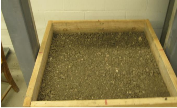
Figure 4.2.3 Unreinforced confined RAP
