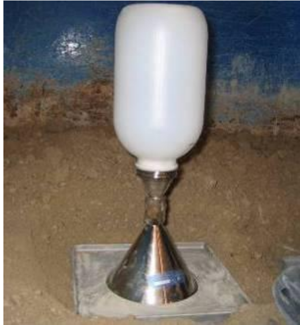
Figure 5.2.7 Sand cone test
