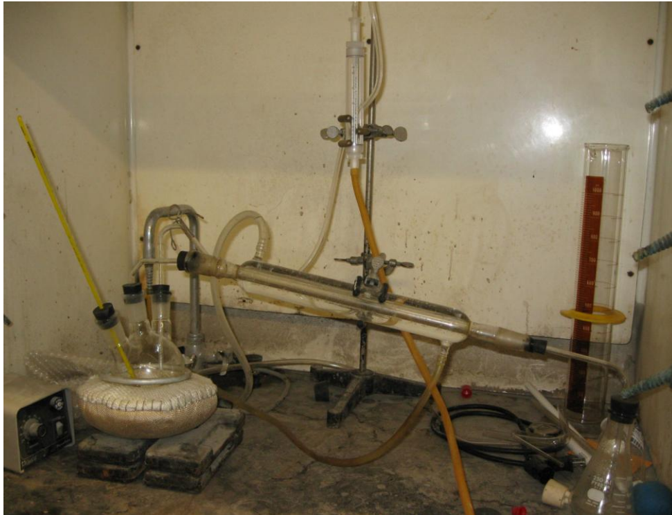
Figure 3.2.12 Set up for asphalt binder recovery by the Abson method
