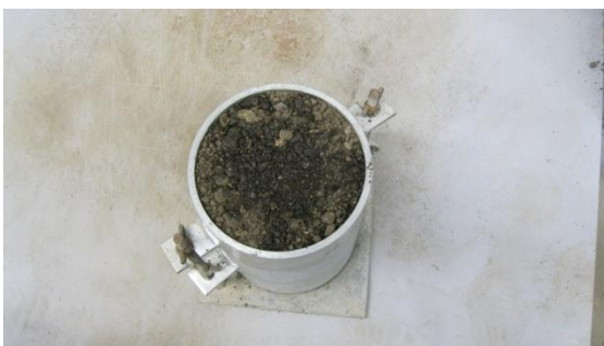
Figure 4.2.7 Fully confined RAP in a compaction mold
