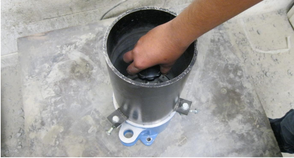
(c) Placing the surcharge base plate on top of the mold
