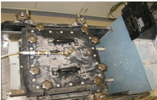
(e) Placing and tightening the top plate and connecting the air pressure hose
