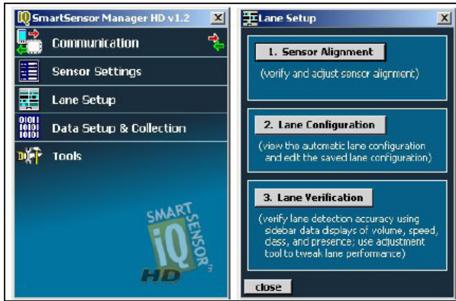
Figure 36 Data Extraction from Smartsensor Using IQ Smartsensor
