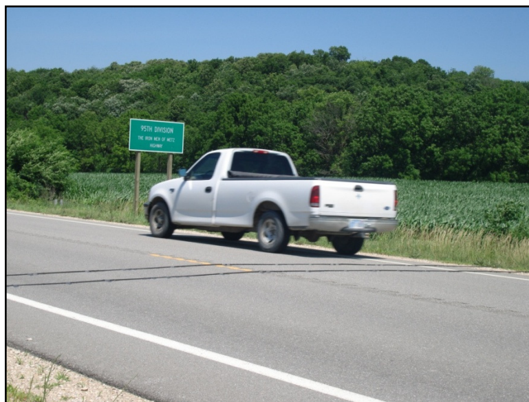
Figure 24 Pneumatic Tubes Laid on Road
