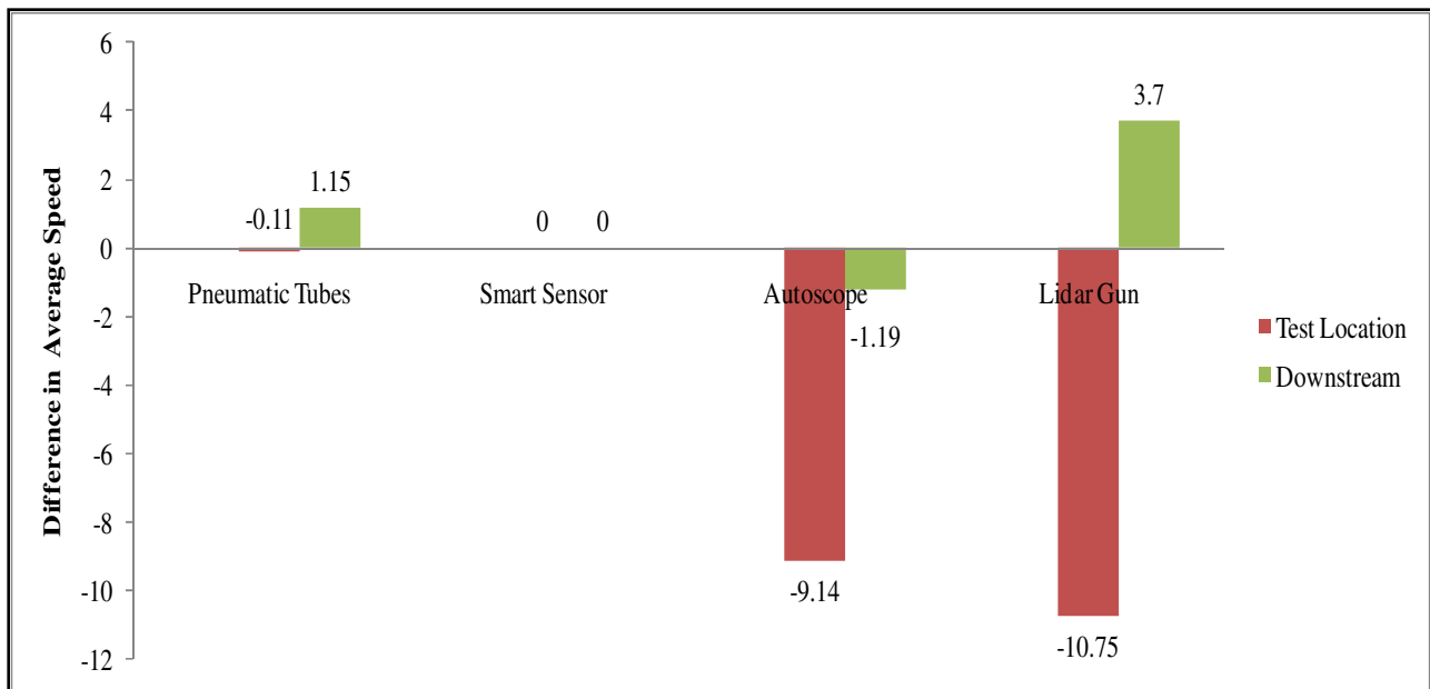
Figure 43 Summary of Difference in Speed Distribution of Fastest 15 Percent Drivers Compared to the Upstream Location
