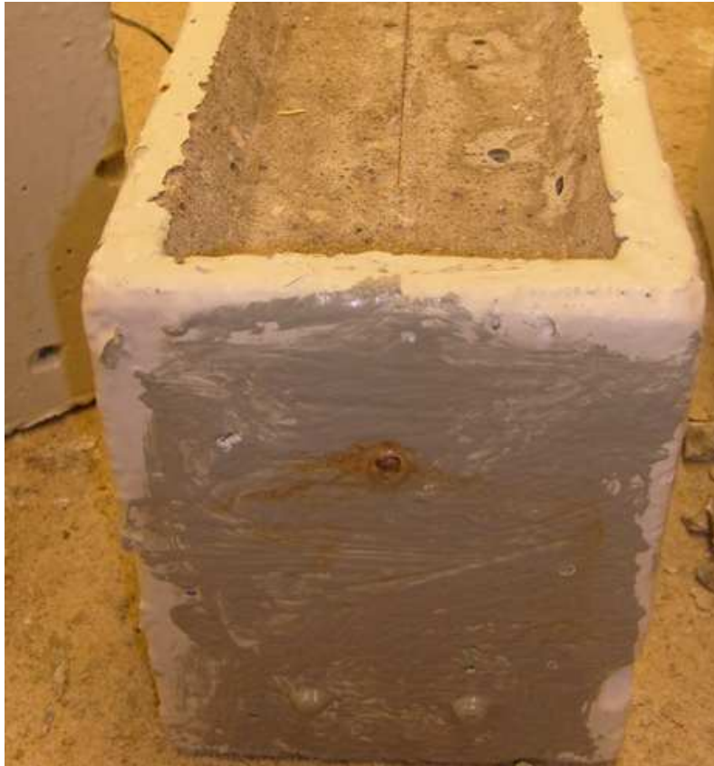
Figure 3.119: CB-MCB(2205p)-5, 240 weeks. Staining at bar ends.
