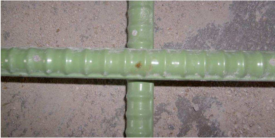
Figure 3.77: FTS-ECR-C-2, showing blistering of the epoxy coating.
