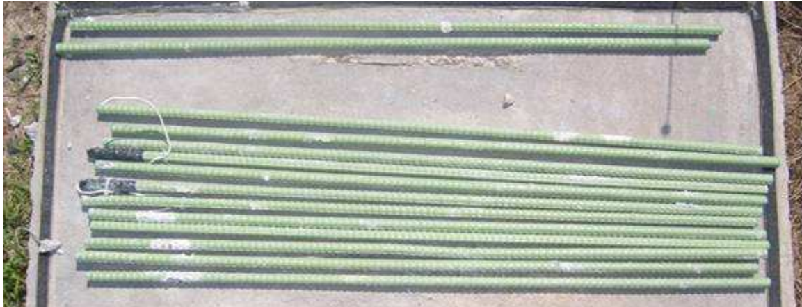
Figure 3.74: FTS-ECR(Chromate)-U-1, showing no visible corrosion products.
