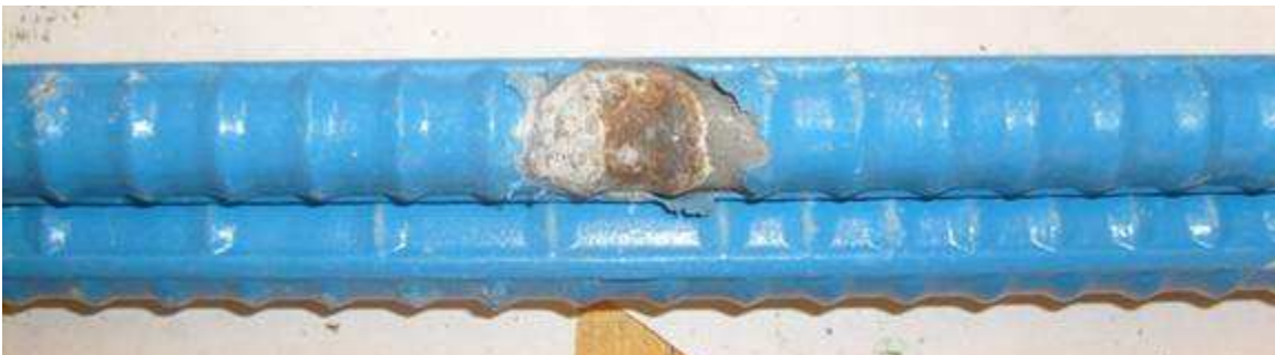
Figure 3.82: FTS-MC-U-2, showing severe disbondment at an intentional damage site.
