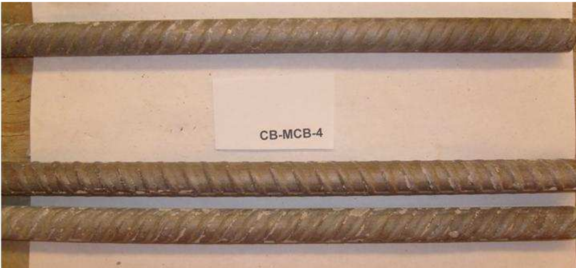
Figure 3.125: CB-MCB(2205p)-4, 240 weeks. No visible corrosion.
