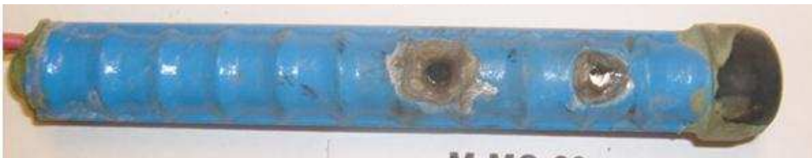
Figure 3.103: Rapid macrocell test, M-MC-23, 40 weeks, after disbondment test.
