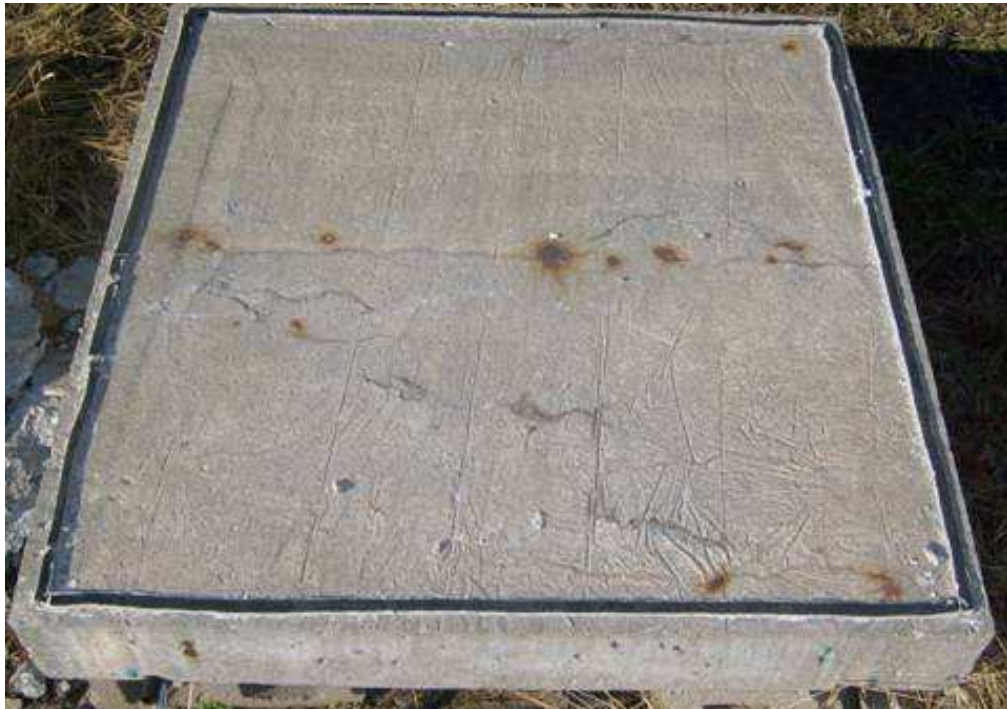
Figure 3.137: Specimen FTS-DCB(Conv.)-1, 240 weeks.
