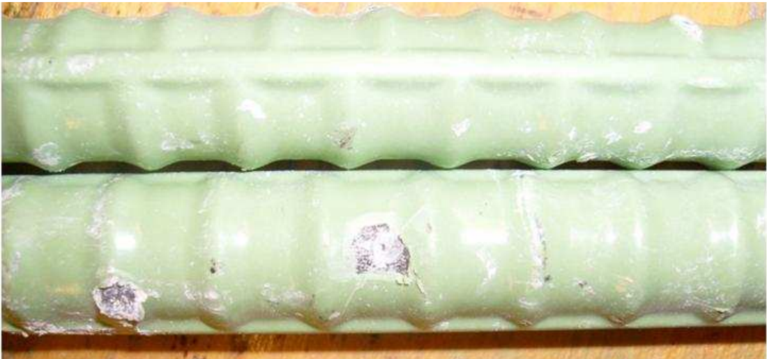
Figure 3.79: FTS-ECR-U-1, showing limited disbondment at an intentional damage site.
