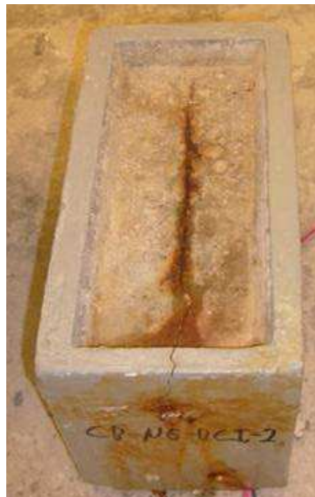
Figure 3.16: Specimen CB-Conv.2-DCI-2, 96 weeks, showing cracking of the concrete.
