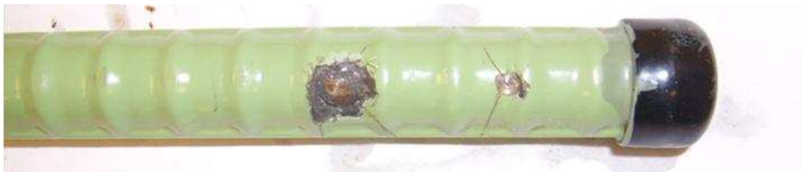
Figure 3.96: Rapid macrocell test, M-ECR-1, 5 weeks, after disbondment test.
