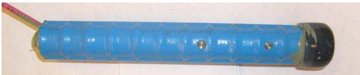
Figure 3.99: Rapid macrocell test, M-MC-4, 10 weeks, before disbondment test.
