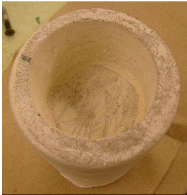
Figure 2.12: Core After Milling
