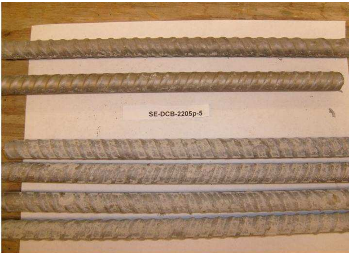
Figure 3.122: SE-DCB(2205p)-5, 240 weeks. Top mat above label, bottom mat below label. No visible corrosion.
