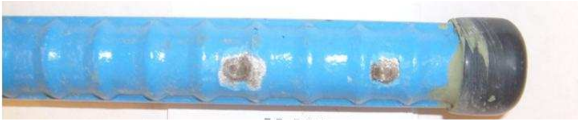
Figure 3.100: Rapid macrocell test, M-MC-4, 10 weeks, after disbondment test.
