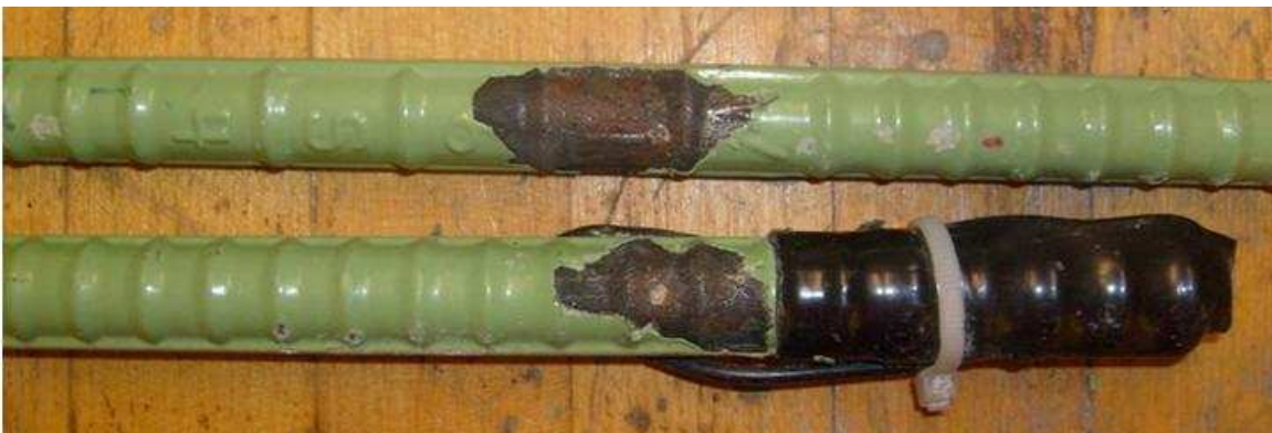
Figure 3.81: FTS-RH-U-2, showing severe disbondment at intentional damage sites.
