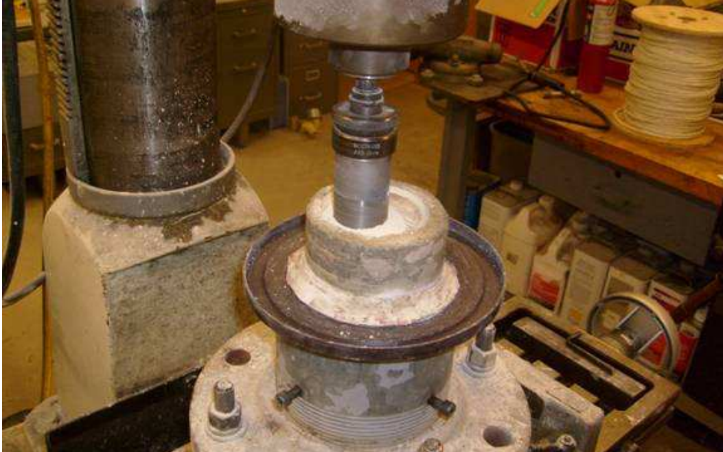
Figure 2.11: Sampling Chlorides from Concrete Core
