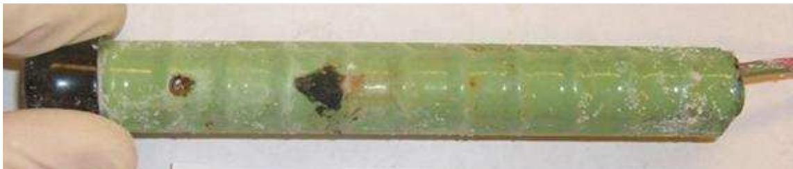
Figure 3.97: Rapid macrocell test, M-ECR-13, 40 weeks, before disbondment test.
