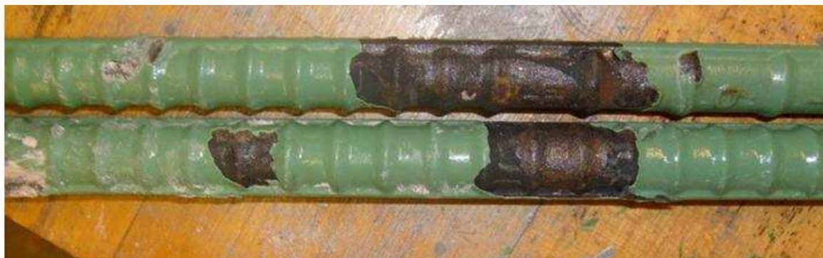
Figure 3.86: FTS-ECR(DuPont)-C-1, showing total disbondment on bars from the top mat of steel.
