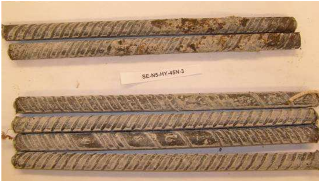
Figure 3.10: Specimen SE-Conv.2-HY-3, 96 weeks. Steel in top mat (above label) and bottom mat (below label).
