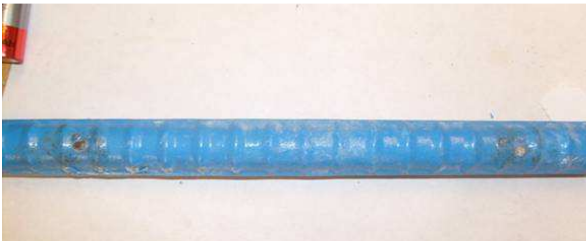
Figure 3.76: FTS-MC-C-2, showing staining at an intentional damage site.
