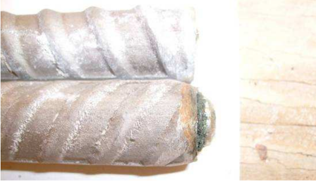
Figure 3.121: SE-MCB(2205p)-5, 240 weeks. Corrosion at ends of top bar.
