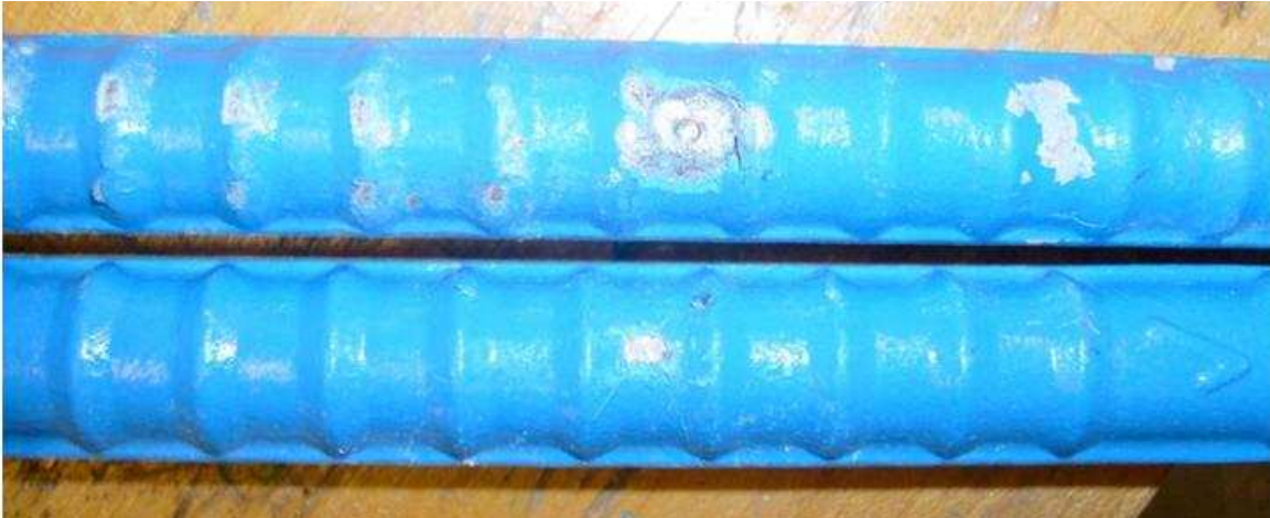
Figure 3.80: FTS-MC-U-1, showing limited disbondment at an intentional damage site.
