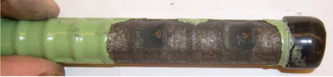
Figure 3.98: Rapid macrocell test, M-ECR-21, 35 weeks, after disbondment test.
