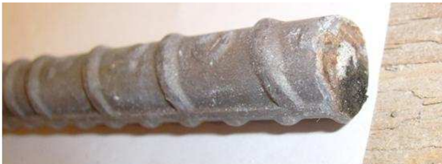
Figure 3.124: CB-MCB(2205p)-2, 240 weeks. Corrosion at bar end.
