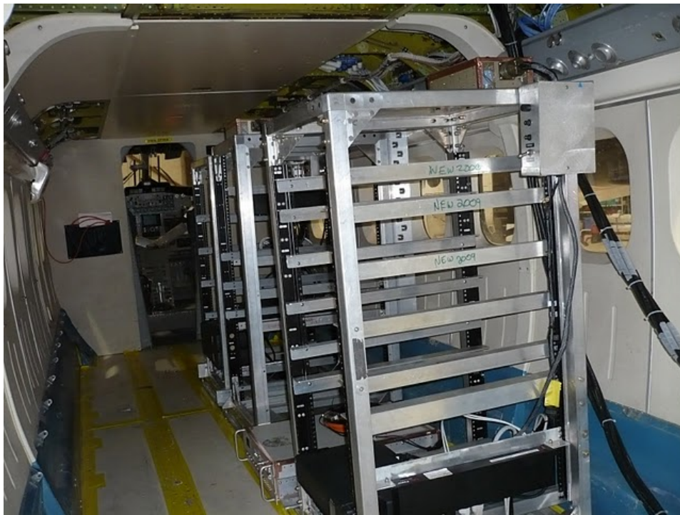
Figure 62. Photograph of the installed empty equipment racks inside the Twin Otter aircraft. Nearest rack houses the accumulation radar and KU-band altimeter.
