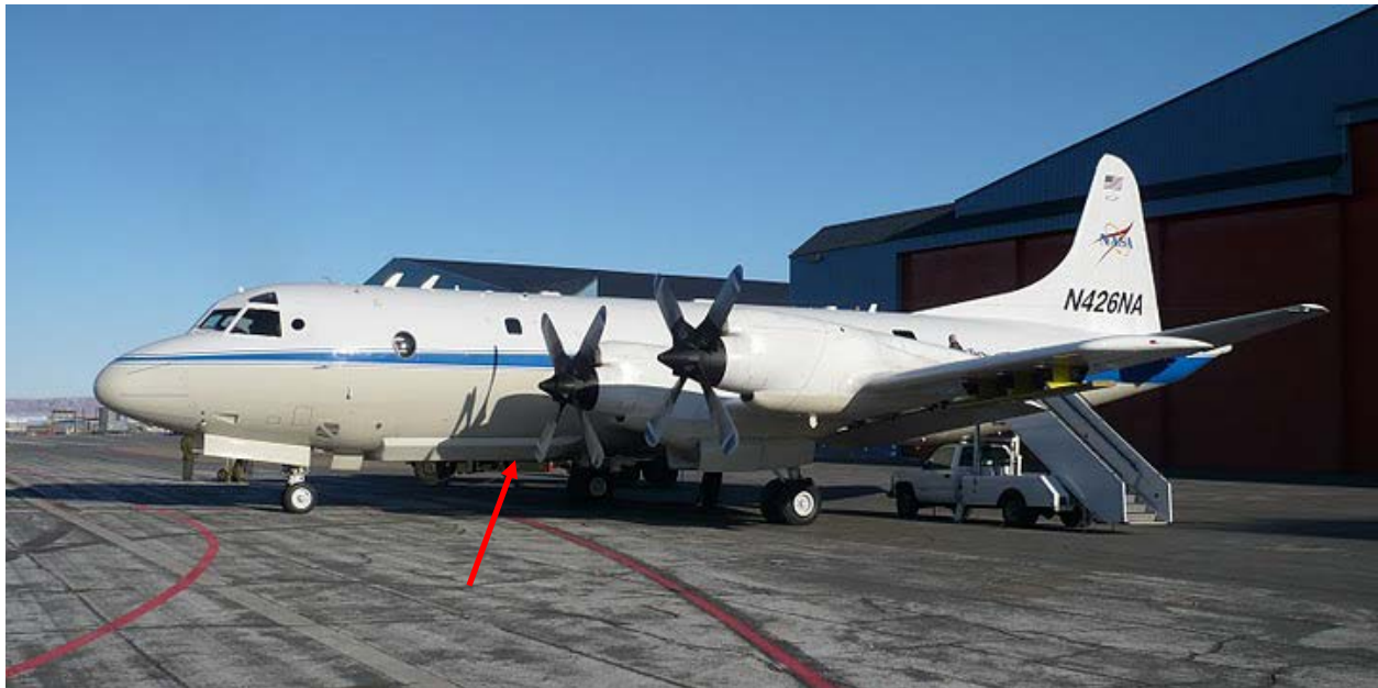
Figure 70. P-3 Orion on the apron at Thule Air Base in northern Greenland. Red arrow indicates the approximate position of the accumulation radar antenna array within the forward bomb bay.
