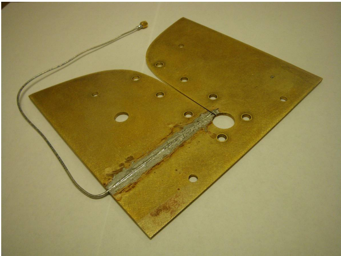
Figure 43. Photograph of the manufactured all-metal Vivaldi (material: brass).
