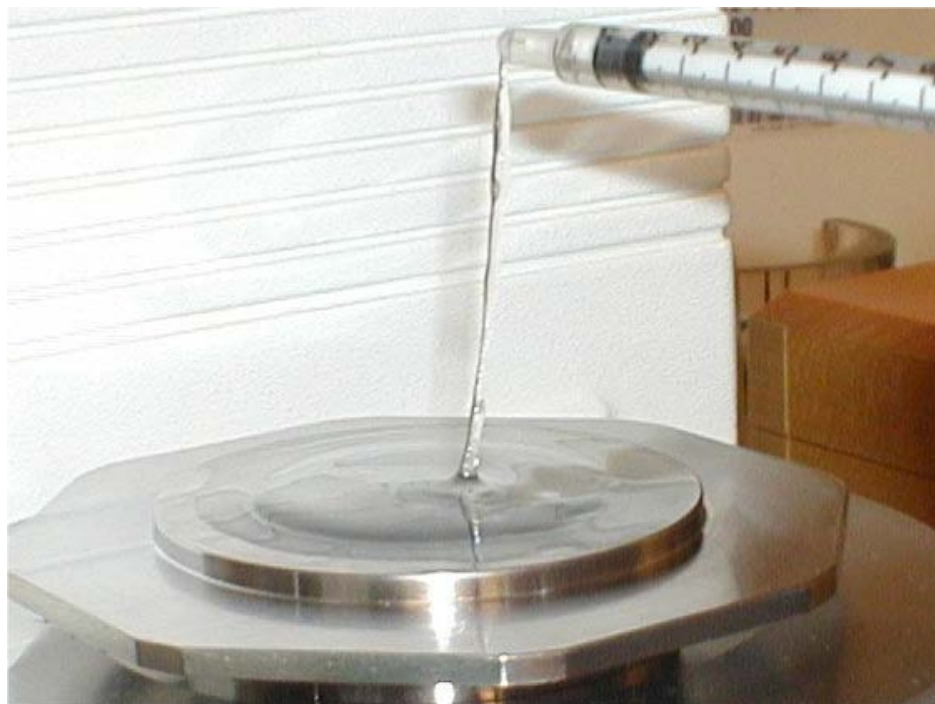
Figure 4.3 Elasticity of sample g050223 after sheared at a constant rate of 110 \text{ s}^{-1} for 10 hours at 41 \text{ }^\circ\text{C}
