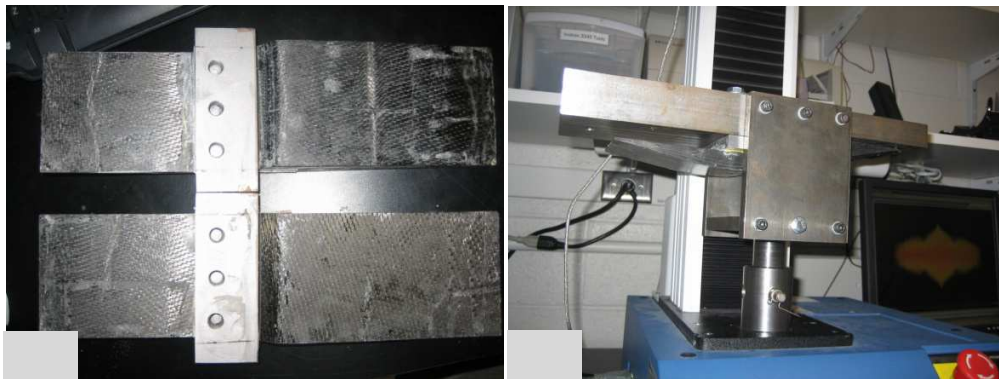
Figure 6: Composite Overlays Attached to Steel Plate: (a) Diagram of Loading Apparatus, (b) Steel Plates Bonded to Composite Overlays, (c) Reaction Apparatus Installed in Testing Machine.
