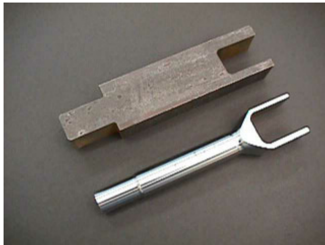
The part on the top was roughed out with a waterjet, with secondary machining creating the part shown on the bottom
