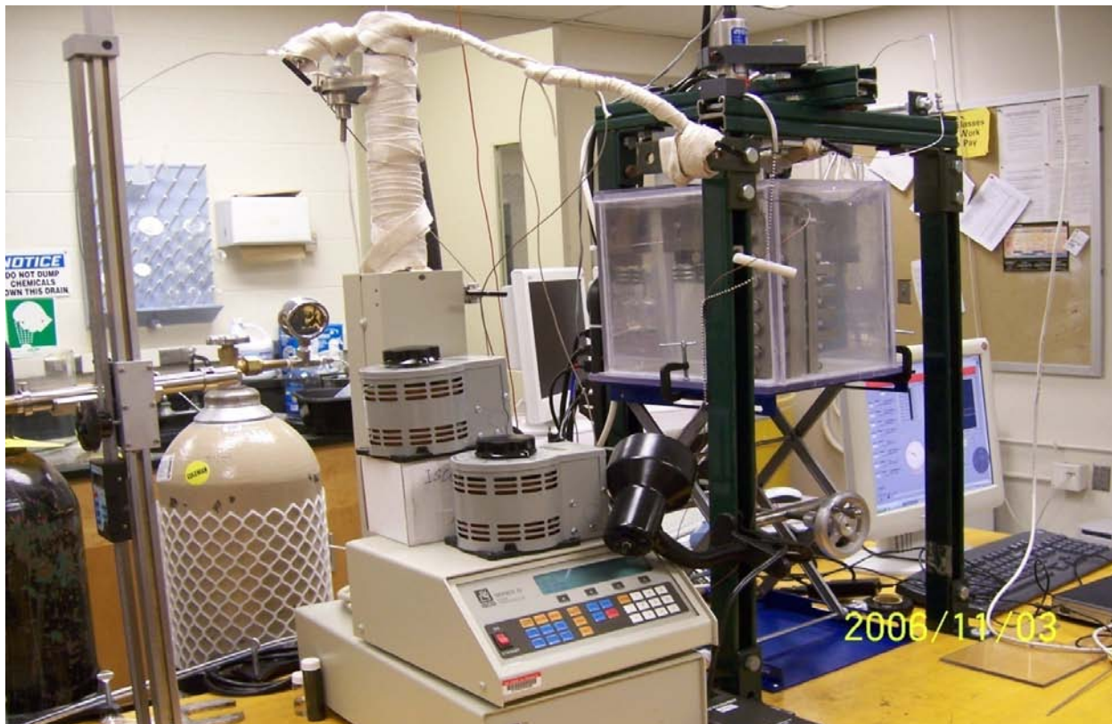
Figure 2-11 An actual image of the swelling/extraction experimental setup
